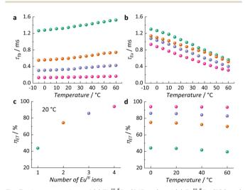
Fig. 3 Average  $\tau$  values of (a) Tb<sup>III 5</sup>D<sub>4</sub> (545 nm) and (b) Eu<sup>III 5</sup>D<sub>0</sub> (700 nm) emitting states of  $\{Eu_1Tb_{19}\}$  (1) (green),  $\{Eu_2Tb_{18}\}$  (2) (orange),  $\{Eu_3Tb_{17}\}$  (3) (purple) and  $\{Eu_4Tb_{16}\}$  (4) (pink) MCAs, as well as  $Tb^{III} \rightarrow Eu^{III}$  ET efficiency  $(\eta)$  at (c) 20 °C and (d) variable temperatures.
