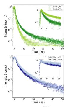
Fig. 3 Time-resolved photoluminescence (TRPL) dynamics of neat PNC films and PC $\subset$ PNCs. PL decay traces of: (A) CsPbBr<sub>3</sub> NCs ( $\lambda_{ex}$  = 390 nm). (B) CsPbCl<sub>1.5</sub>Br<sub>1.5</sub> NCs ( $\lambda_{ex} = 350 \text{ nm}$ ).
