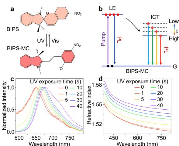
**Fig. 1** (a) Reversible photoisomerization of BIPS between spirobypyan and merocyanine forms. (b) Energy diagram for the concentration-dependent ICT process of BIPS-MC. (c) PL spectra from a 20 wt% BIPS@PMMA film at different UV exposure times. (d) Refractive indices of the BIPS@PMMA film with increasing exposure time to UV light.
