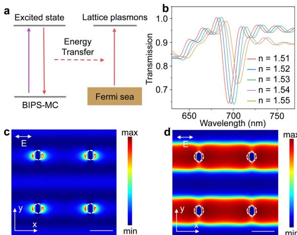
**Fig. 2** (a) Energy diagram for the coupling between the BIPS-MC and the lattice plasmons. (b) FDTD-simulated transmission spectra of the Ag nanoparticle array in different dielectric environments ( $n = 1.51\text{--}1.55$ ). (c) FDTD-simulated distribution map of electric field intensity ( $|E|^2$ ) of the Ag nanoparticle array at the  $x$ - $y$  plane. (d) FDTD-simulated phase distribution map of the Ag nanoparticle array at the  $x$ - $y$  plane. Scale bars in (c) and (d): 200 nm.
