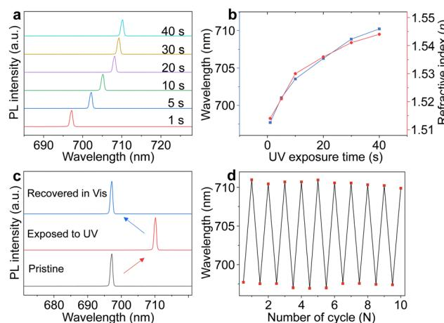
**Fig. 4** (a) Time-dependent lasing spectra of the BIPS@PMMA film-covered Ag nanoparticle array on exposure to UV light. (b) Plots of the lasing wavelength and refractive index of the BIPS@PMMA film-covered Ag nanoparticle array *versus* time of exposure to UV light. (c) Lasing spectra of the BIPS@PMMA film-covered Ag nanoparticle array under alternate irradiation with UV and Vis light. (d) Plot of the lasing wavelength *versus* switching cycles.
