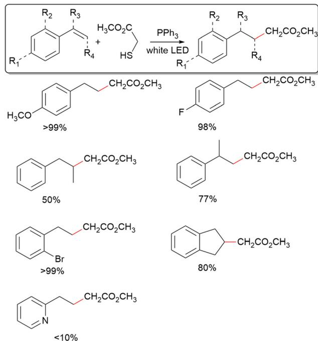
Reaction conditions: 0.4 mmol of styrene derivatives, 157 mg b-TPP, 72  $\mu$ L b-2, 2 mL acetonitrile (solvent), 0.8 W cm<sup>-2</sup> (Dolan–Jenner Fiber-Lite MI-LED B1), photoillumination for 18 hours, no atmospheric control, and 60 °C. All reactions were run without a stir bar to avoid contamination. Reaction yields were determined using <sup>1</sup>H-NMR with *t*-cinnamaldehyde as internal standard.
