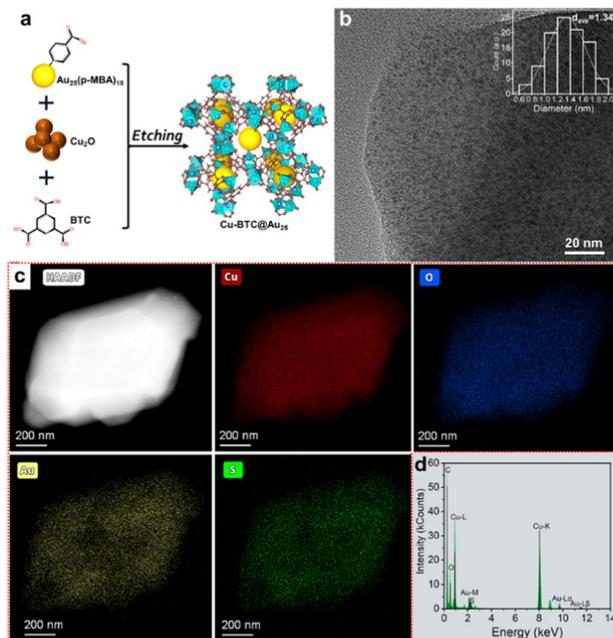
Fig. 1 (a) Schematic illustration of the preparation process of the  $\text{Au}_{25}$ @Cu-BTC composite. (b) HRTEM image, (c) STEM image and corresponding EDS elemental mapping images and (d) EDS spectrum of  $\text{Au}_{25}$ @Cu-BTC.
