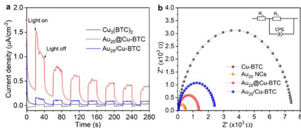
Fig. 3 (a) Photocurrents and (b) Nyquist plots of  $\text{Cu}_3(\text{BTC})_2$ , Au NCs,  $\text{Au}_{25}@\text{Cu-BTC}$  and  $\text{Au}_{25}/\text{Cu-BTC}$ . The inset in (b) is the equivalent circuit for fitting.
