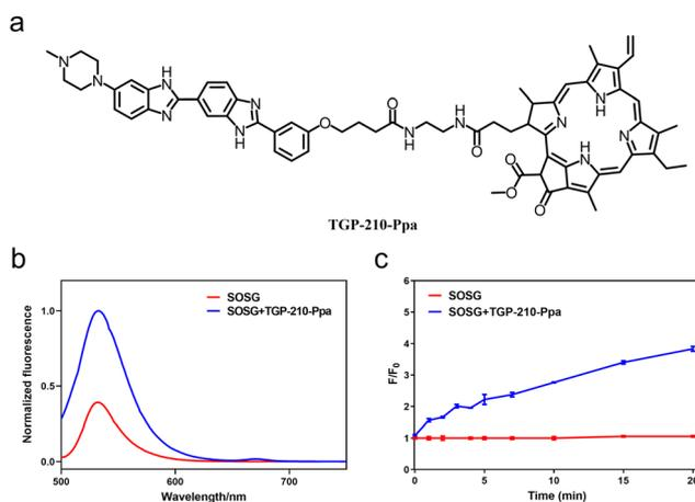
**Fig. 1** (a) Chemical structure of **TGP-210-Ppa**. (b) Fluorescence spectra of **TGP-210-Ppa** after irradiation with 670 nm light ( $70 \text{ mW cm}^{-2}$ ) for 5 min. (c) The increase of SOSG fluorescence at 530 nm after incubation with **TGP-210-Ppa** and irradiation by 670 nm light ( $70 \text{ mW cm}^{-2}$ ) for 0–20 min.  $\lambda_{\text{ex}} = 488 \text{ nm}$ . Data are shown as mean  $\pm$  SEM ( $n = 3$ ).
