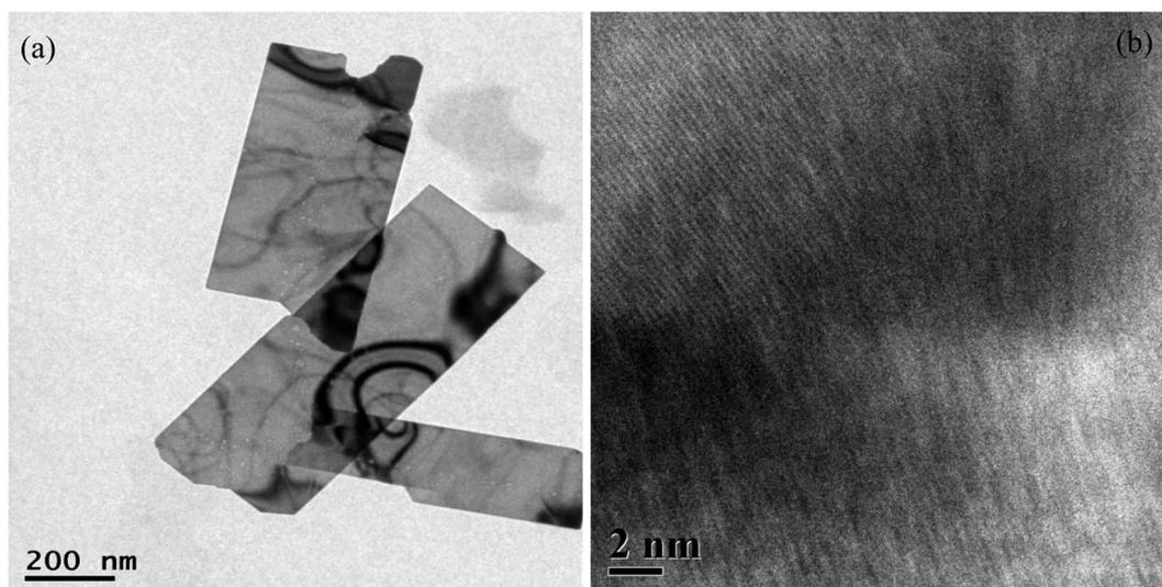
Fig. 2 (a) TEM and (b) HRTEM images of Cu nanosheets.
