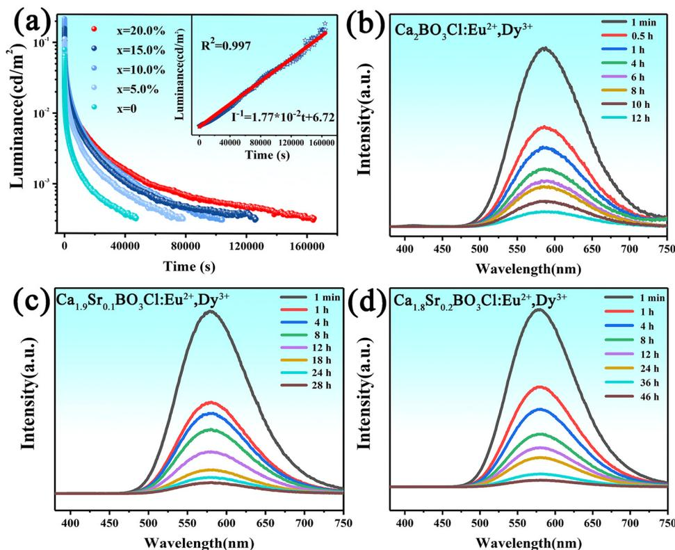
Fig. 3 (a) Afterglow decay curves of the  $\text{Ca}_{2-x}\text{Sr}_x\text{BO}_3\text{Cl}:\text{Eu}^{2+},\text{Dy}^{3+}$  series of samples (the inset indicates the inverse of the afterglow intensity *versus* time for  $\text{Ca}_{1.8}\text{Sr}_{0.2}\text{BO}_3\text{Cl}:\text{Eu}^{2+},\text{Dy}^{3+}$ ) and (b–d) afterglow spectra of  $\text{Ca}_{2-x}\text{Sr}_x\text{BO}_3\text{Cl}:\text{Eu}^{2+},\text{Dy}^{3+}$  ( $x = 0, 10\%, 20\%$ ).
