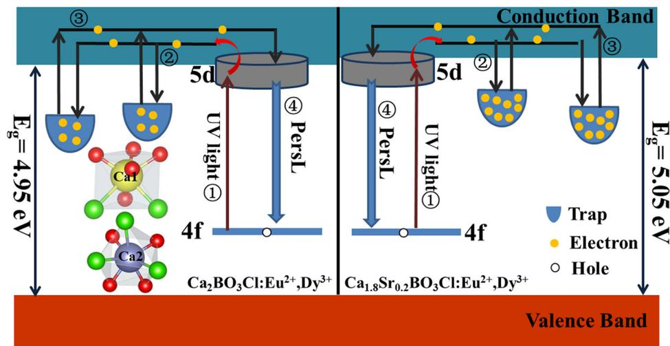
Fig. 5 The schematic diagram of the PersL mechanism of  $\text{Ca}_2\text{BO}_3\text{Cl}:\text{Eu}^{2+},\text{Dy}^{3+}$  and  $\text{Ca}_{1.8}\text{Sr}_{0.2}\text{BO}_3\text{Cl}:\text{Eu}^{2+},\text{Dy}^{3+}$ .
