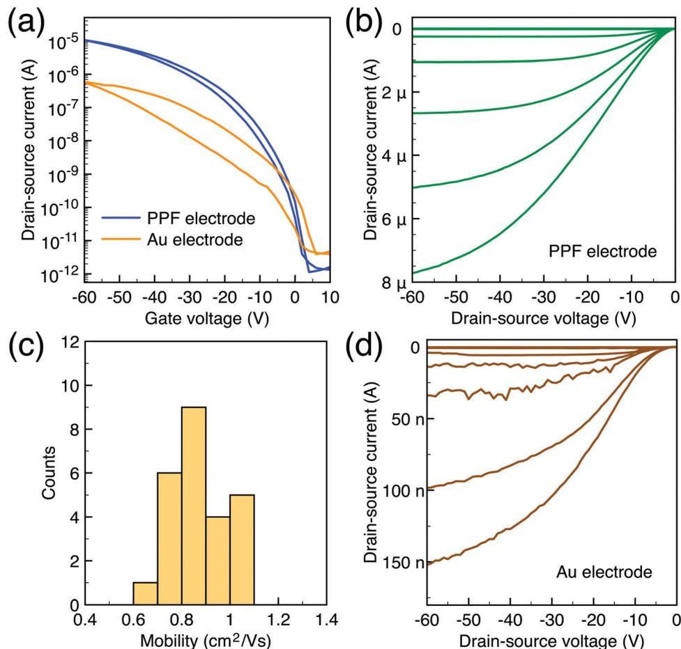
Fig. 4 (a) Transfer  $I$ - $V$  curve of DNTT transistors based on PPF and Au electrodes. (b) Output  $I$ - $V$  curve of DNTT transistors based on PPF electrodes; the  $V_{\text{G}}$  voltage step is 10 V. (c) Mobility histogram of 25 devices. (d) Output  $I$ - $V$  curve of DNTT transistors based on Au electrodes; the  $V_{\text{G}}$  voltage step is 10 V.
