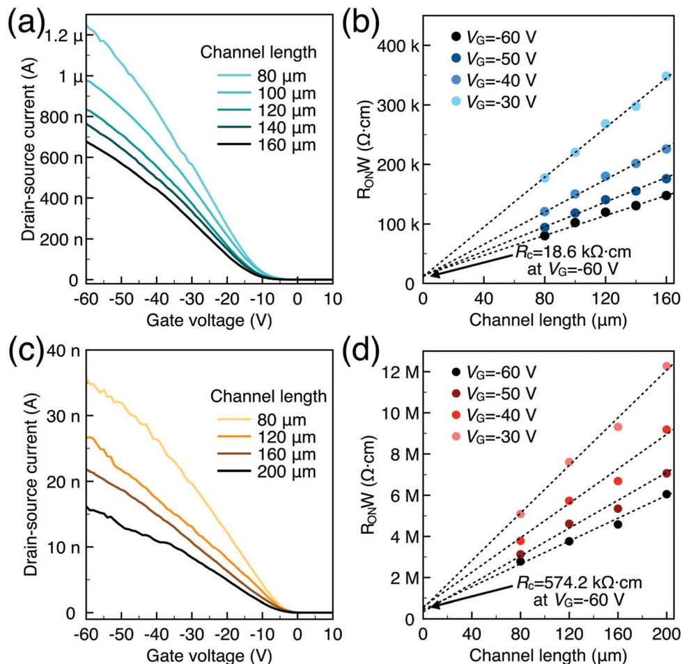
Fig. 5 (a) Transfer  $I$ - $V$  of carbon-based OFETs; (b) contact resistance of carbon-based OFETs at various  $V_G$ ; (c) transfer  $I$ - $V$  of Au-based OFETs; (d) contact resistance of Au-based OFETs at various  $V_G$ .
