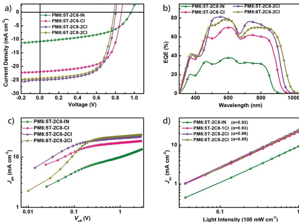
**Fig. 2** (a)  $J$ – $V$  curves of **PM6:5T-2C8-IN/5T-2C8-Cl/5T-2C8-2Cl** and **PM6:6T-2C8-2Cl** based devices under one sun illumination (AM 1.5G 100 mW cm<sup>-2</sup>). (b) EQE spectra of the corresponding devices. (c)  $J_{ph}$  versus  $V_{eff}$  and (d) light-intensity ( $P$ ) dependence of  $J_{sc}$  measurement of the devices.
