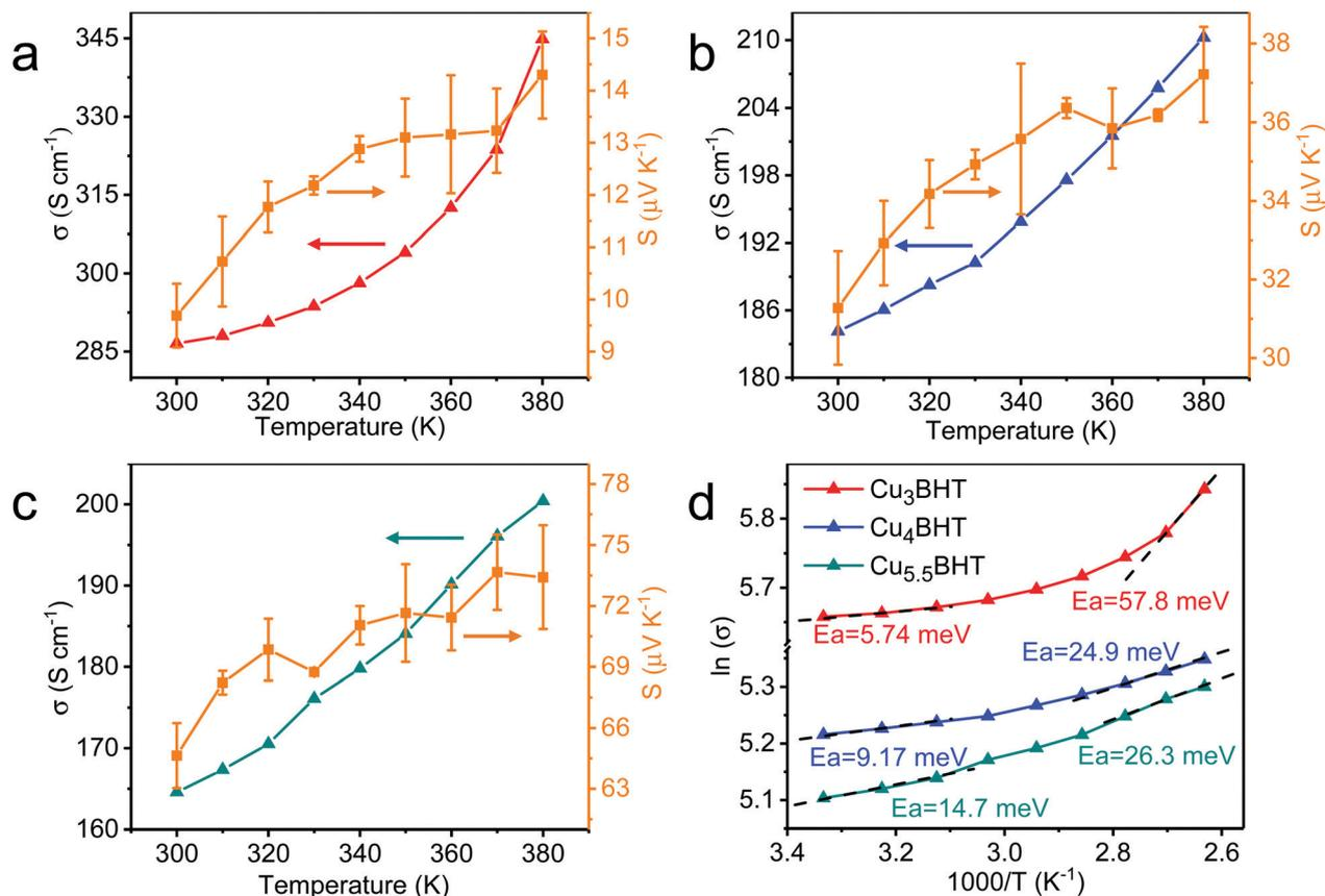
Fig. 3 The charge transport properties of Cu<sub>x</sub>BHT. (a–c) Curves of the variable-temperature electrical conductivity and Seebeck coefficient of Cu<sub>3</sub>BHT, Cu<sub>4</sub>BHT and Cu<sub>5.5</sub>BHT, respectively. (d) Plots of  $\ln(\sigma T)$  versus  $1000/T$  of Cu<sub>x</sub>BHT.
