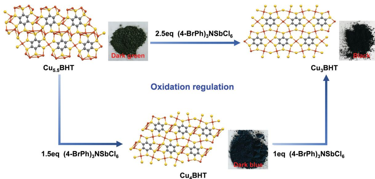
Fig. 5 Oxidation regulation within the  $\text{Cu}_x\text{BHT}$  family. Schematic illustration of phase transition in  $\text{Cu}_x\text{BHT}$  species upon delicate oxidation regulation with  $(4\text{-BrPh})_3\text{NSbCl}_6$ . Photograph shows the colours of each  $\text{Cu}_x\text{BHT}$  species.
