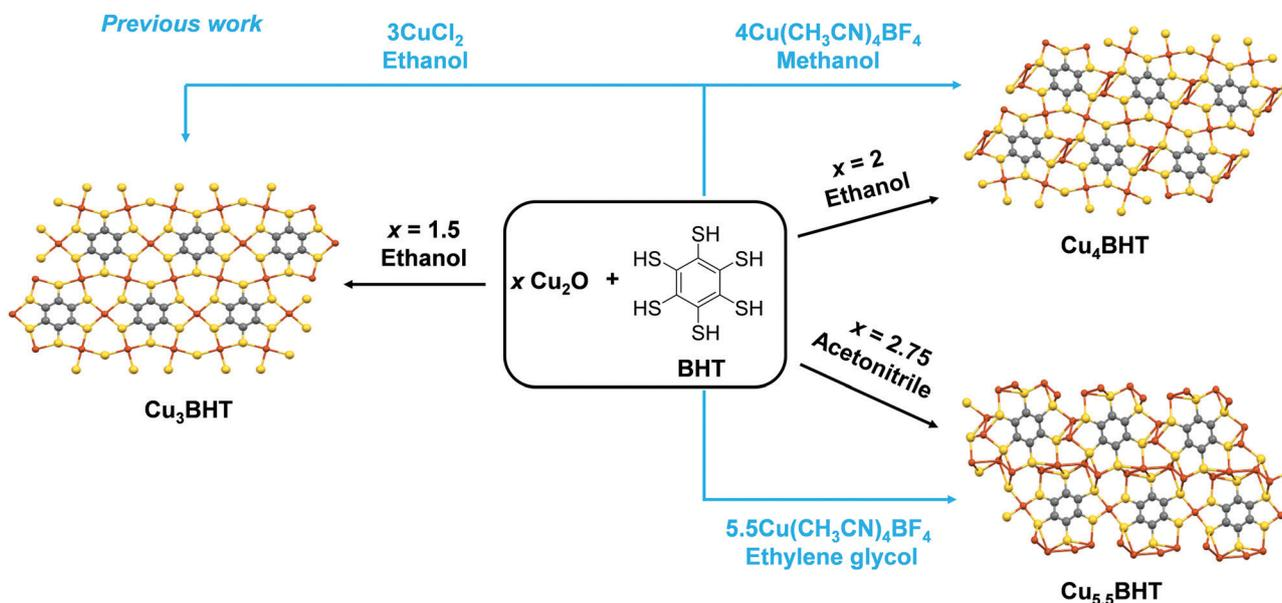
Fig. 1 Comparison of the synthetic methods of  $\text{Cu}_x\text{BHT}$  ( $x = 3, 4,$  and  $5.5$ ). The schematic synthesis of  $\text{Cu}_x\text{BHT}$  using different metal sources and reaction solvents. The previously reported pathways (ref. 13 and 16) are indicated by blue lines and text.
