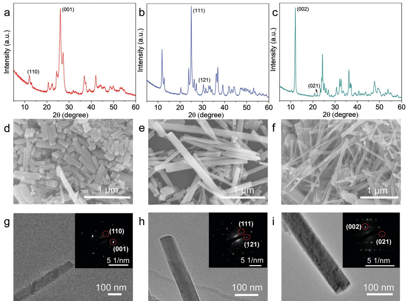
Fig. 2 Characterization of  $\text{Cu}_x\text{BHT}$ . (a–c) PXRD patterns of  $\text{Cu}_3\text{BHT}$ ,  $\text{Cu}_4\text{BHT}$  and  $\text{Cu}_{5.5}\text{BHT}$ , respectively. (d–f) SEM images of  $\text{Cu}_3\text{BHT}$ ,  $\text{Cu}_4\text{BHT}$  and  $\text{Cu}_{5.5}\text{BHT}$ , respectively. (g–i) TEM images of  $\text{Cu}_3\text{BHT}$ ,  $\text{Cu}_4\text{BHT}$  and  $\text{Cu}_{5.5}\text{BHT}$ , respectively. Insets correspond to SAED patterns.
