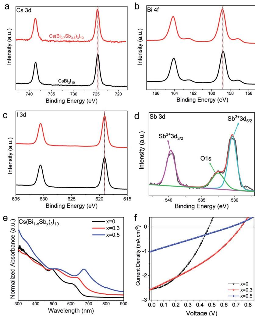
**Fig. 2** XPS spectra of (a) Cs 3d, (b) Bi 4f, and (c) I 3d of CBI and CBSI-3 films, and (d) Sb 3d of CBSI-3 film. (e) UV-vis spectra of CBI, CBSI-3, and CBSI-5 films on the ITO/PEDOT substrate. (f)  $J$ - $V$  curves of CBI, CBSI-3, and CBSI-5 devices with an inverted device architecture (ITO/PEDOT/CSBI/PCBM/bathocuproine (BCP)/Ag) measured under illumination (AM 1.5G, 100 mW cm<sup>-2</sup>). All films illustrated here are synthesized from DMF/DMSO mixed solvent with volume ratio of 9 : 1.
