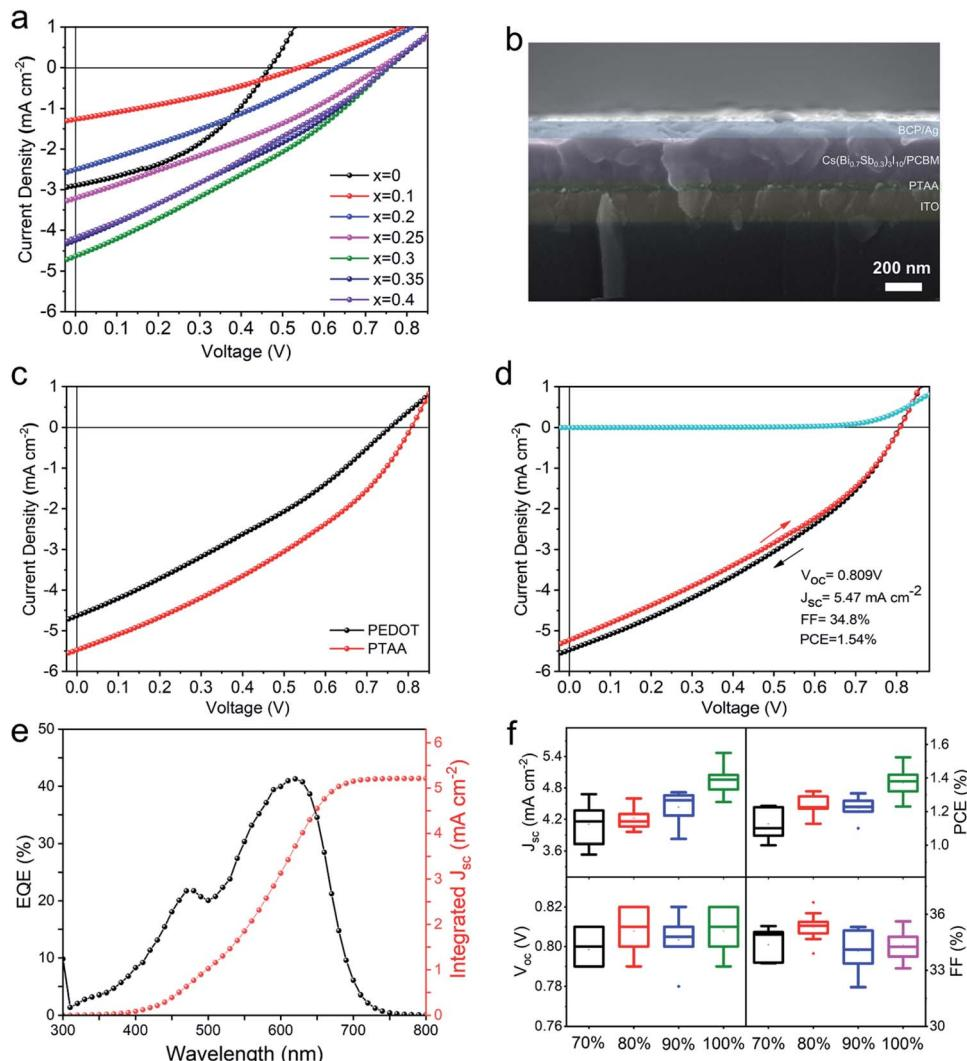
**Fig. 4** (a)  $J$ – $V$  curves of CBSI-based solar cells with different Sb substitution by using pure 100 vol% DMSO as the solvent. (b) Cross-sectional SEM image of the CBSI-3 solar cell by using PTAA as the HTL. (c)  $J$ – $V$  curves of the CBSI-3 solar cells with PEDOT or PTAA as the HTL. (d)  $J$ – $V$  and (e) EQE curves of the champion CBSI-3 solar cell. (f) Statistic variations of CBSI-3 devices fabricated by using solvents with different DMSO volume ratios.
