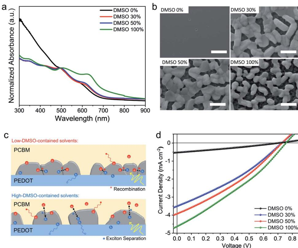
**Fig. 3** (a) UV-vis spectra, (b) SEM images of CBSI-3 films synthesized from DMF/DMSO mixed solvents with different DMSO volume ratios. (c) Proposed exciton separation and charge transfer processes for CBSI-3 films synthesized from low- or high-DMSO-contained solvents. (d) The corresponding  $J$ - $V$  curves of CBSI-3 based solar cells with the structure of ITO/PEDOT/CBSI-3/PCBM/BCP/Ag measured under illumination (AM 1.5G, 100 mW  $\text{cm}^{-2}$ ).
