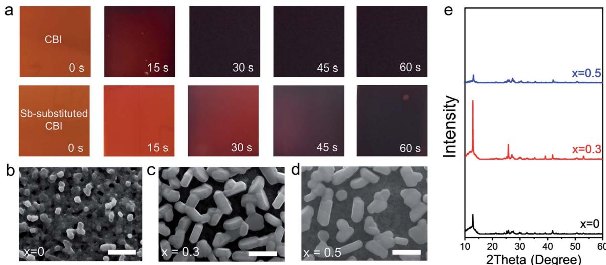
**Fig. 1** (a) Photographs of  $\text{CsBi}_3\text{I}_{10}$  (CBI) and  $\text{Cs}(\text{Bi}_{1-x}\text{Sb}_{0.3})_x\text{I}_{10}$  (CBSI-3) films with different thermal annealing duration. SEM images of (b) CBI, (c) CBSI-3, and (d) CBSI-5 films, the scale bar corresponds to 500 nm. (e) XRD patterns of CBI ( $x = 0$ ), CBSI-3 ( $x = 0.3$ ), and CBSI-5 ( $x = 0.5$ ) films. (All films illustrated here are synthesized from DMF/DMSO mixed solvent with the volume ratio of 9 : 1).
