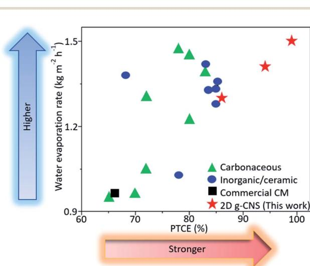
Fig. 5 Comparison of solar vapor generation performances of 2D g-CNS solar evaporators with previously reported solar evaporators under one-sun illumination (see details in Table S1, ESI†).
