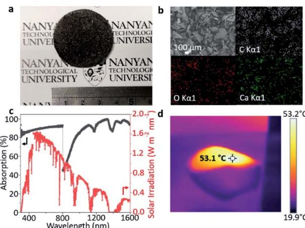
Fig. 3 (a) Photograph of 2D g-CNS<sub>PB</sub> deposited on air-laid paper, (b) FESEM image of a 2D g-CNS<sub>PB</sub> photothermal layer with its corresponding EDX mapping images of C, O and Ca elements, (c) UV-vis-NIR absorption spectrum of 2D g-CNS<sub>PB</sub> with AM 1.5 solar irradiance as a reference. (d) Thermal image of the 2D g-CNS<sub>PB</sub> photothermal layer under air.
