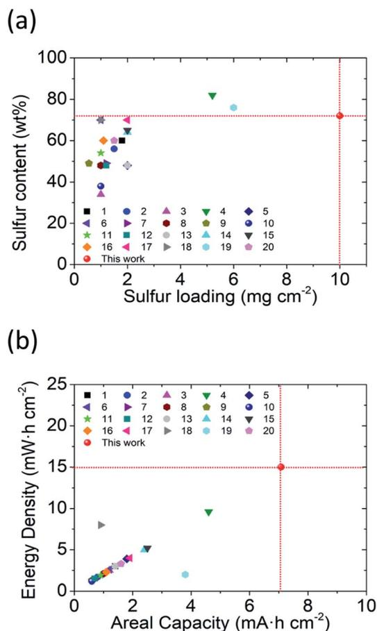
Fig. 5 Comparison of the cell-design parameters and cell-electrochemical performances of lithium-sulfur batteries with the PMMA-based GPE and other GPEs: (a) sulfur loading ( $\text{mg cm}^{-2}$ ) and content (wt%) and (b) areal capacity ( $\text{mA h cm}^{-2}$ ) and energy density ( $\text{mW h cm}^{-2}$ ) based on the whole electrode.
