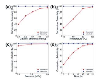
Fig. 6 Effect of various reaction parameters on the cycloaddition of CO2 and ECH with MOF-801(D) catalysts (a) catalyst amount (cocatalyst 0.5 mol%, 80 °C, 15 h, 0.1 MPa CO<sub>2</sub>), (b) temperature (catalyst 0.6 mol%, co-catalyst 0.5 mol%, 15 h, 0.1 MPa CO<sub>2</sub>), (c) CO<sub>2</sub> pressure (catalyst 0.6 mol%, co-catalyst 0.5 mol%, 80 °C, 15 h), and (d) time (catalyst 0.6 mol%, co-catalyst 0.5 mol%, 80 °C, 0.1 MPa CO<sub>2</sub>).
