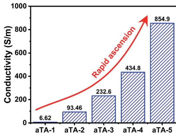
Fig. 4 Histogram of the conductivity of anisotropic aerogels with different MXene contents.
