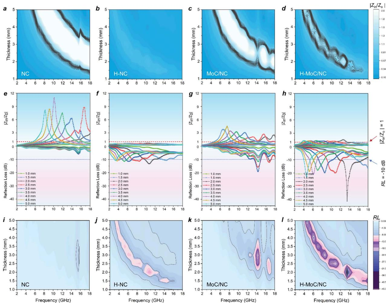
Fig. 4 (a–d) 2D contour map of  $|Z_{in}/Z_0|$  for NC, H-NC, MoC/NC and H-MoC/NC. (e–h) The  $|Z_{in}/Z_0|$  and RL plots of NC, H-NC, MoC/NC and H-MoC/NC. (i–l) 2D contour map of RL for NC, H-NC, MoC/NC and H-MoC/NC.
