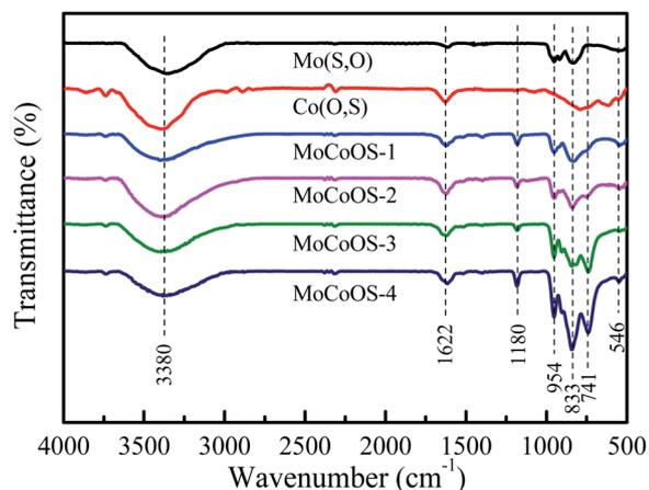
Fig. 3 FTIR spectra of Mo(S,O), Co(O,S), and MoCoOS prepared with different amounts of  $\text{CoCl}_2 \cdot 6\text{H}_2\text{O}$ .
