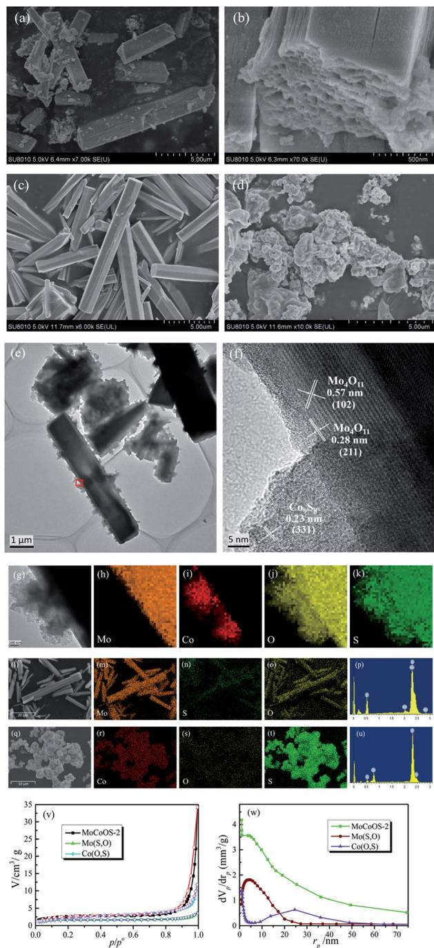
**Fig. 4** (a and b) SEM images of MoCoOS-2. SEM images of (c) Mo(S,O) and (d) Co(O,S). (e) TEM and (f) HR-TEM images of MoCoOS-2. (g–k) EDX element distribution mapping images of Mo, Co, O, and S for MoCoOS-2. (l–p) EDX element distribution mapping images of Mo, O, and S for Mo(S,O). (q–u) EDX element distribution mapping images of Co, O, and S for Co(O,S). (v) Nitrogen adsorption–desorption isotherm and (w) the pore size distribution curve of the catalysts.
