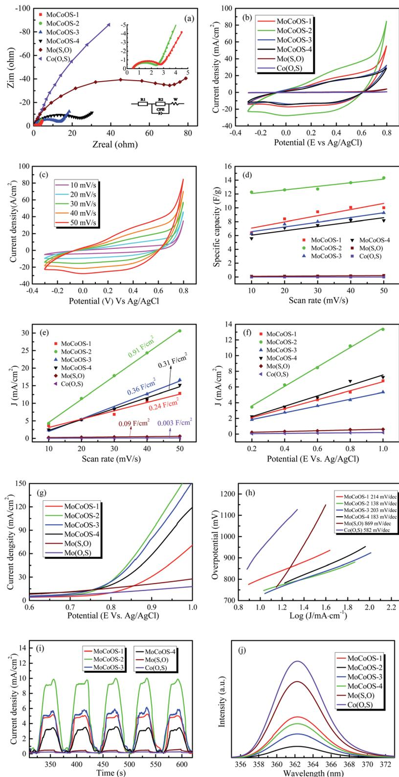
**Fig. 6** (a) Electrochemical impedance spectra of MoCoOS with different Co contents. (b) Current density of different MoCoOS under  $50 \text{ mV s}^{-1}$  scan rate. (c) Current density of MoCoOS-2 under different scan rates. (d) Specific capacity of MoCoOS under different scan rates. The variations of current density with (e) scan rate and (f) different voltages. (g) LSV, (h) Tafel curves, (i) transient photocurrent (TPC), and (j) PL spectra of Mo(S,O), Co(O,S), and MoCoOS catalysts.
