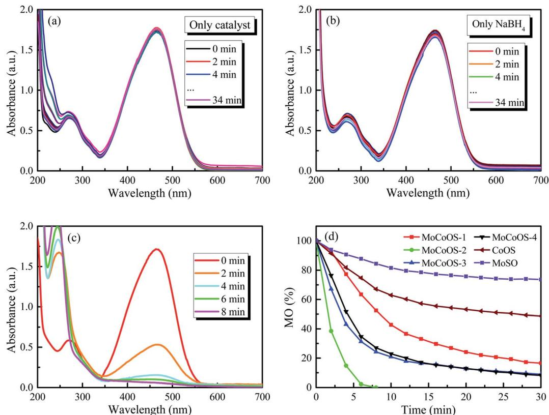
Fig. 9 (a) Reduction of MO with only MoCoOS-2. (b) Reduction of MO with only NaBH<sub>4</sub>. (c) Reduction of MO with MoCoOS-2 and NaBH<sub>4</sub>. (d) Reduction of MO with Mo(S,O), Co(O,S), and MoCoOS catalysts in the presence of NaBH<sub>4</sub>.
