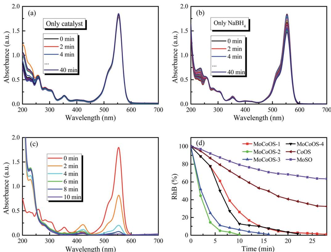
Fig. 11 (a) Reaction of RhB with only MoCoOS-2. (b) Reaction of RhB with only NaBH<sub>4</sub>. (c) Reduction of RhB with MoCoOS-2 and NaBH<sub>4</sub>. (d) Reduction of RhB with Mo(S,O), Co(O,S), and MoCoOS catalysts in the presence of NaBH<sub>4</sub>.
