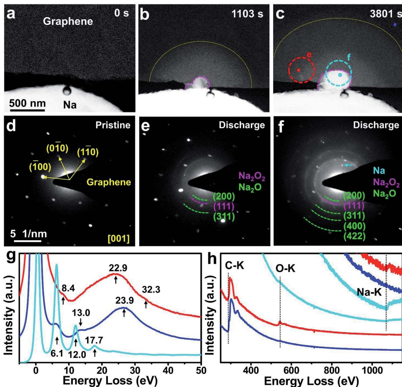
Fig. 3 *In situ* TEM observation and characterization of an Na–O<sub>2</sub> nanobattery with a multilayered graphene cathode. (a–c) Time-lapse structural evolution of the graphene cathode in an Na–O<sub>2</sub> nanobattery during the discharge process. (d–f) EDPs and (g, h) EELS of the pristine graphene and discharge products on the graphene cathode. The blue and cyan/red dots correspond to the unreacted and reacted regions, respectively.
