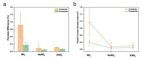
Fig. 5 In the equivalent reaction setup as in Fig. 3 with Cu catalysts and  $NO_2^-$  (0.5 M) or  $NO_3^-$  (1 M) in place of  $NH_3$  at -0.98 V vs. RHE, formamide and acetamide were generated. The faradaic efficiencies (a) and partial current densities (b) for their generation were compared to those from using NH<sub>3</sub>.
