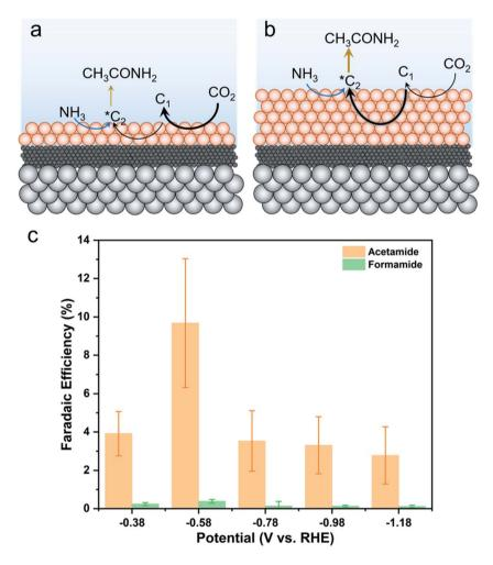
Fig. 6 A thicker catalyst loading was found to promote acetamide formation. Thin layers tend to form C<sub>1</sub> products at a greater rate (a) while increasing the layer thickness leads to further reduction and accumulation of C2 intermediates that can be used for C-N bond formation (b). As such, an optimized Cu loading of 10 mg cm<sup>-2</sup> resulted in up to 10% acetamide selectivity (c).
