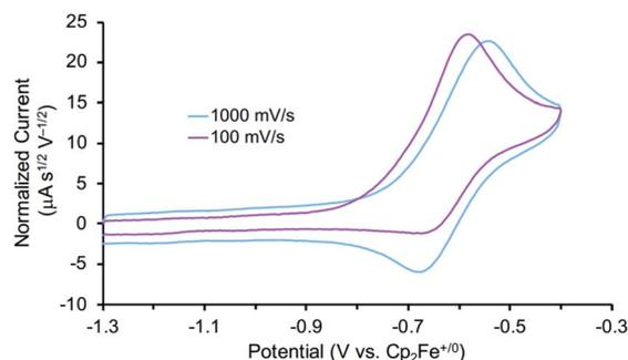
**Fig. 3** Cyclic voltammogram of the first oxidation of **3** (0.2 mM) in 0.2 M NBu<sub>4</sub>PF<sub>6</sub> solution in THF under N<sub>2</sub> using a glassy carbon working electrode, Pt wire auxiliary electrode, and Ag wire pseudoreference. Potentials referenced to Cp<sub>2</sub>Fe<sup>+0</sup> after the experiments.
