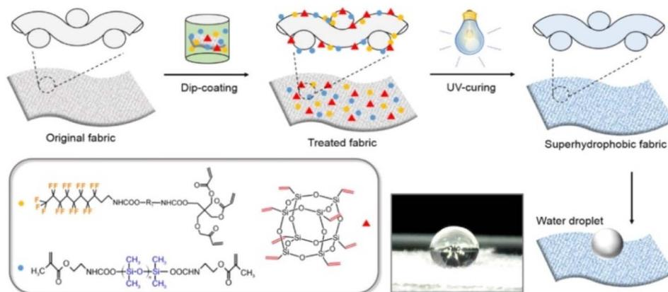
Fig. 12 Preparation of UV curable superhydrophobic self-healing textile coating. This figure has been adapted from ref. 58 with permission from Elsevier, copyright 2017.
