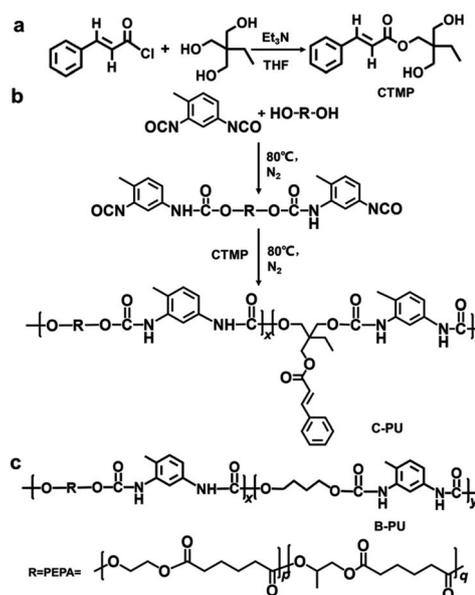
Fig. 9 Synthesis of photocrosslinkable polyurethane containing cinnamoyl. This figure has been adapted from ref. <sup>53</sup> with permission from Royal Society of Chemistry, copyright 2019.
