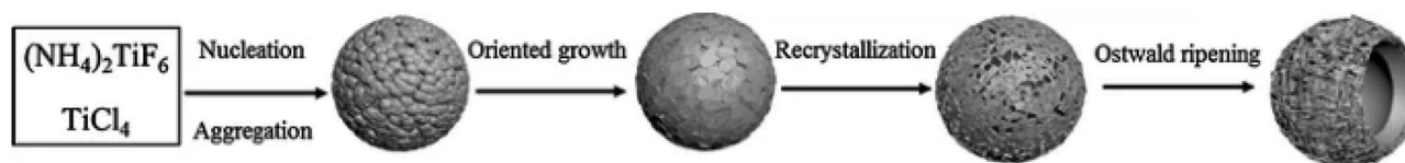
Fig. 6 Schematic illustration of the probable formation mechanism of hollow porous \text{TiO}_2 microspheres. 97
