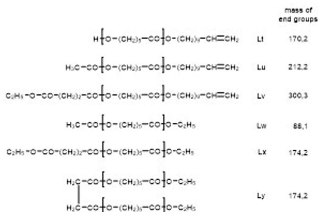
Scheme 5 Potential reaction products of the transesterifications of AcPCLUn with DESu catalyzed by neat TSA.
