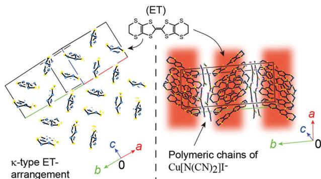
Fig. 1 Crystal structure of **1**. Blue, violet, yellow, orange, and green spheres represent C, N, S, Cu, and I atoms, respectively. The H atoms were omitted for clarity. Two-dimensional conduction pathways are highlighted in red.
