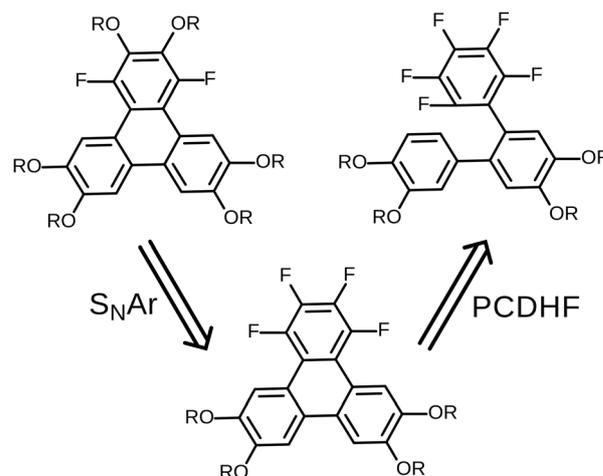
**Scheme 2** Retrosynthetic analysis for fluorinated alkoxytriphenylenes. The viability of this synthesis approach requires regioselectivity in both of the S<sub>N</sub>Ar and PCDHF steps.
