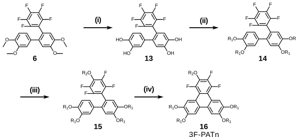
**Scheme 7** The synthesis of pentakisalkoxytriphenylene discotic liquid crystals. (i)  $\text{BBr}_3/\text{DCM}$ ,  $\sim 100\%$ ; (ii)  $\text{R}_1\text{-I}/\text{K}_2\text{CO}_3/\text{DMF}$ , 68% for  $\text{R}_1 = \text{C}_6\text{H}_{13}$ ; (iii)  $\text{R}_2\text{-OH}/t\text{-BuOK}$ , 70% for  $\text{R}_2 = \text{C}_6\text{H}_{13}$ ; (iv) PCDHF, 55% for  $\text{R}_1 = \text{R}_2 = \text{C}_6\text{H}_{13}$ .
