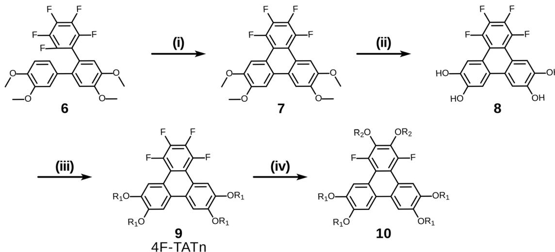
**Scheme 5** The synthesis of hexakisalkoxytriphenylene discotic liquid crystals. (i) PCDHF, 89%; (ii)  $\text{BBr}_3/\text{DCM}$ , 98%; (iii)  $\text{R}_1\text{-I}/\text{K}_2\text{CO}_3/\text{DMF}$ , 87% for  $\text{R}_1 = \text{C}_6\text{H}_{13}$ ; (iv)  $\text{R}_2\text{-OH}/t\text{-BuOK}$ , 58% for  $\text{R}_2 = \text{C}_6\text{H}_{13}$ , 81% for  $\text{R}_2 = \text{C}_{12}\text{H}_{25}$ .
