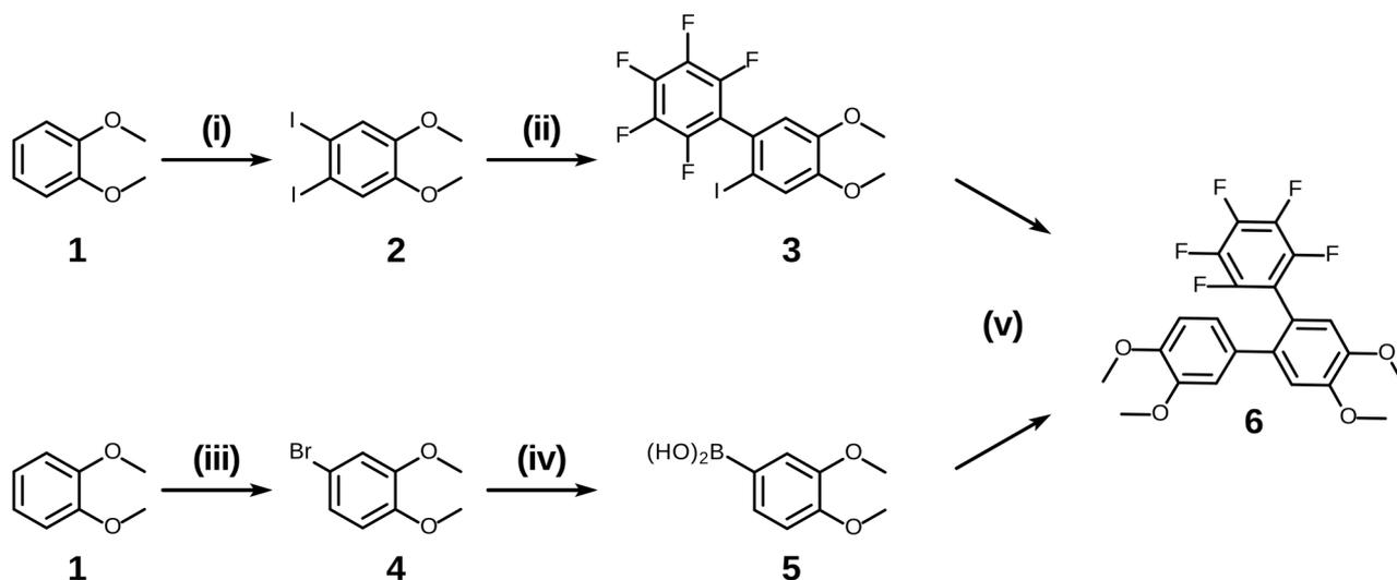
**Scheme 4** The synthesis of *o*-terphenyl intermediate **6**. (i)  $\text{I}_2$ /periodic acid/methanol, 89%; (ii)  $\text{PhF}_5\text{COOK}/\text{CuI}$  (0.1 eq.)/diglyme/ $150^\circ\text{C}$ , 55%; (iii)  $\text{NBS}/\text{silica Gel}/\text{CHCl}_3/\text{rt}$ , 92%; (iv) (1)  $n\text{-BuLi}/-78^\circ\text{C}$ , (2) triisopropyl borate/ $-78^\circ\text{C}$ , (3)  $\text{HCl}/\text{rt}$ , 51%; (v)  $\text{Pd}(\text{PPh}_3)_4/1,4\text{-dioxane}/\text{water}$ , 73%.
