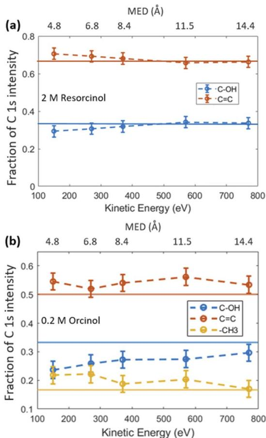
Fig. 2 (a) The fractional contribution of aromatic carbon ( $\text{C}=\text{C}$ , red) and carboxylic carbon ( $\text{C}-\text{OH}$ , blue) components to the C 1s photoemission intensity in 2 M RES solution. The blue and red thin lines indicate the theoretical ratio of the carboxylic carbon (33.3%) and aromatic carbon (66.7%), respectively. (b) Fractional contributions of carbons for the 0.2 M ORC case, including the aliphatic carbon contribution ( $\text{C}-\text{CH}_3$ , yellow).
