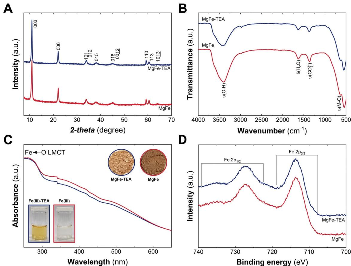
**Fig. 1** Structural and physicochemical characterization of MgFe samples obtained with (blue) and without (red) TEA: PXRD patterns (A); ATR-FTIR and (B) UV-vis diffuse reflectance. (C) The insets depict the digital photographs of iron aqueous solution with and without TEA (Fe(III)-TEA and Fe(III), respectively) and the obtained solids, MgFe-TEA and MgFe; high resolution Fe 2p XPS spectra in the range of 740–700 eV (D).
