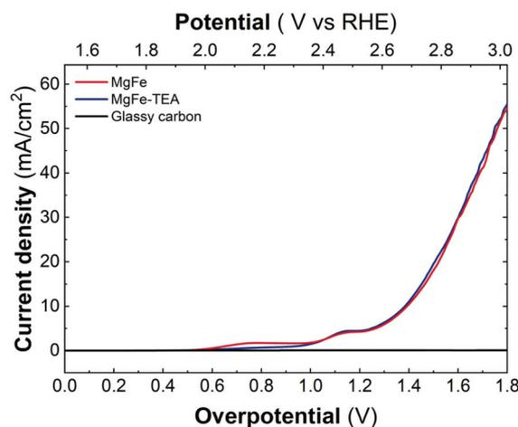
**Fig. 5** Linear sweep voltammetry (LSV) recorded at  $5 \text{ mV s}^{-1}$  in  $1 \text{ M KOH}$  solution by employing glassy carbon collectors for samples obtained with and without TEA, MgFe-TEA (blue) and MgFe (red), in comparison with the bare collector (black).
