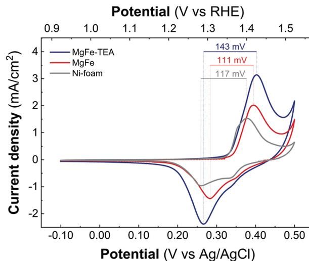
**Fig. 7** Cyclic voltammetry recorded at  $5 \text{ mV s}^{-1}$  between  $-0.1 \text{ V}$  and  $0.4 \text{ V}$  versus Ag/AgCl for the samples MgFe-TEA (blue) and MgFe (red) and Ni-foam (gray) after 20 cycles of the activation process.
