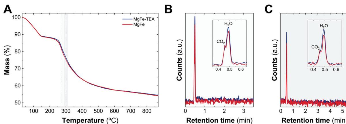
Fig. 2 TG-GC-MS characterization. TG patterns of MgFe-TEA (blue) and MgFe (red) recorded at 10 °C min<sup>-1</sup> under an inert atmosphere of helium (A). During the decomposition process, the evolved gaseous fragments are injected in a preheated GC column at 40 °C. After chromatographic separation, the molecules were identified by MS. Elugrams from the injection at 270 (B) and 300 °C (C) only allow us to identify CO<sub>2</sub> and H<sub>2</sub>O molecules during the decomposition process.
