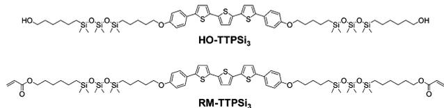
Fig. 1 Chemical structures of terthiophene-siloxane mesogens **HO-TTPSi<sub>3</sub>** and **RM-TTPSi<sub>3</sub>**.
