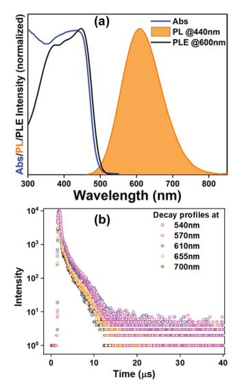
Fig. 2 Optical characterization of (BzTEA)<sub>2</sub>TeCl<sub>6</sub> showing (a) absorbance (Abs), photoluminescence (PL), and photoluminescence excitation (PLE) spectra; (b) lifetime decay profiles collected across the PL band ( $\lambda_{exc}$  = 440 nm).
