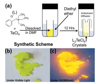
Fig. 1 (a) Reaction scheme (anti-solvent diffusion) utilized for the synthesis of single crystals of (BzTEA)<sub>2</sub>TeCl<sub>6</sub>; photograph of the synthesized crystals at room temperature under (b) visible and (c) UV illumination (365 nm).
