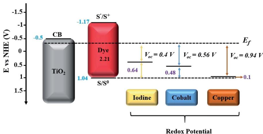
Fig. 5 Energetics in DSSCs with respect to redox potentials of each redox couple ( $I^-/I_3^-$ ,  $[Co(bpy)_3]^{2+/3+}$  and  $[Cu(dmp)_2]^{1+/2+}$ ) utilized in DSSCs.<sup>55</sup>
