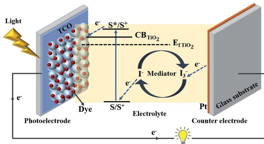
Fig. 2 Schematic illustration representing device structure and working principle of a dye-sensitized solar cell. CB = conduction band,  $E_{fTiO_2}$  = fermi level of  $TiO_2$ , S = ground state of dye sensitizer molecule,  $S^*$  = excited state of dye sensitizer molecule,  $S^0$  = oxidized dye,  $S^+$  = charge separation,  $I^-$  = iodide ion and  $I_3^-$  = triiodide ion.
