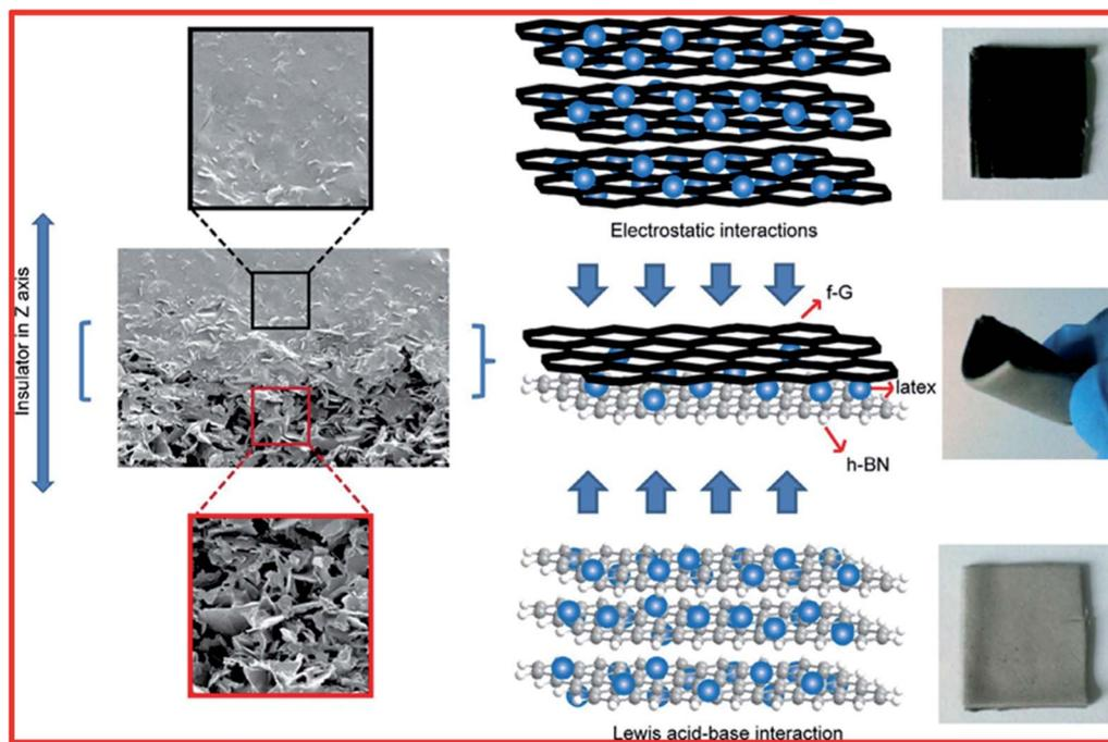
Fig. 25 The laminated structure of a flexible f-G/h-BN composite.<sup>235</sup>
