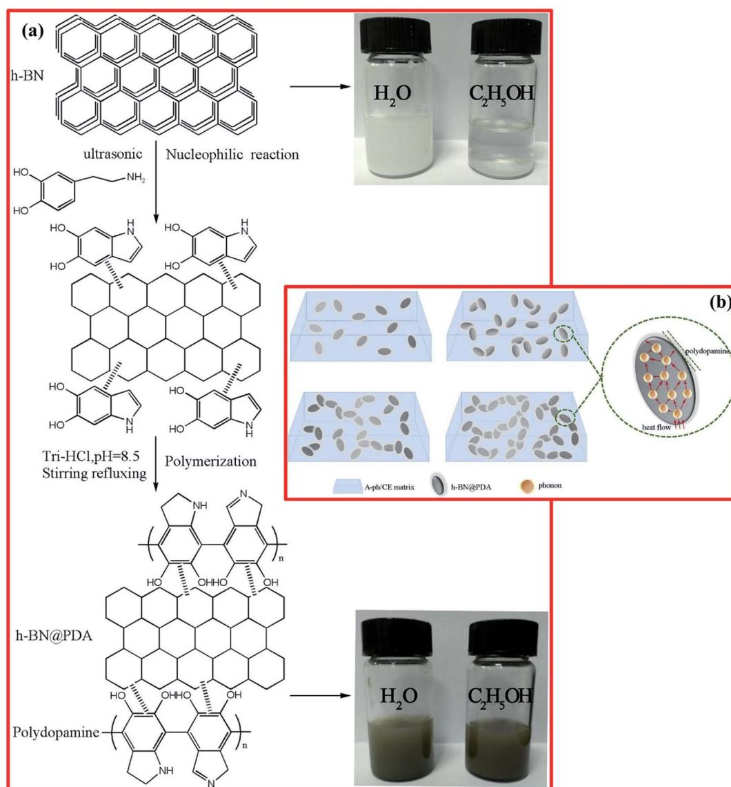
Fig. 24 (a) The reaction mechanism of dopamine-modified h-BN nanoparticles and images of dispersions in ethanol and water. (b) A schematic diagram of the heat-conduction mechanism.<sup>223</sup>
