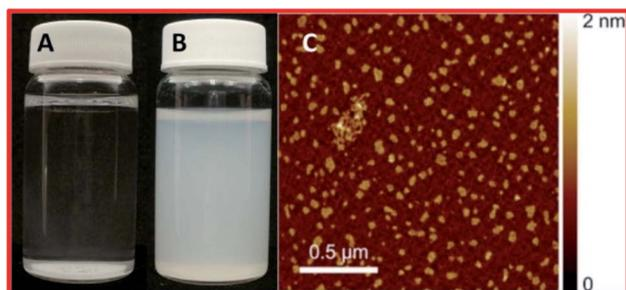
Fig. 9 (A) Unfunctionalized hBN in water, (B) functionalized and exfoliated h-BN in water, and (C) an AFM image of oxidized and exfoliated h-BN nanosheets.<sup>66</sup>
