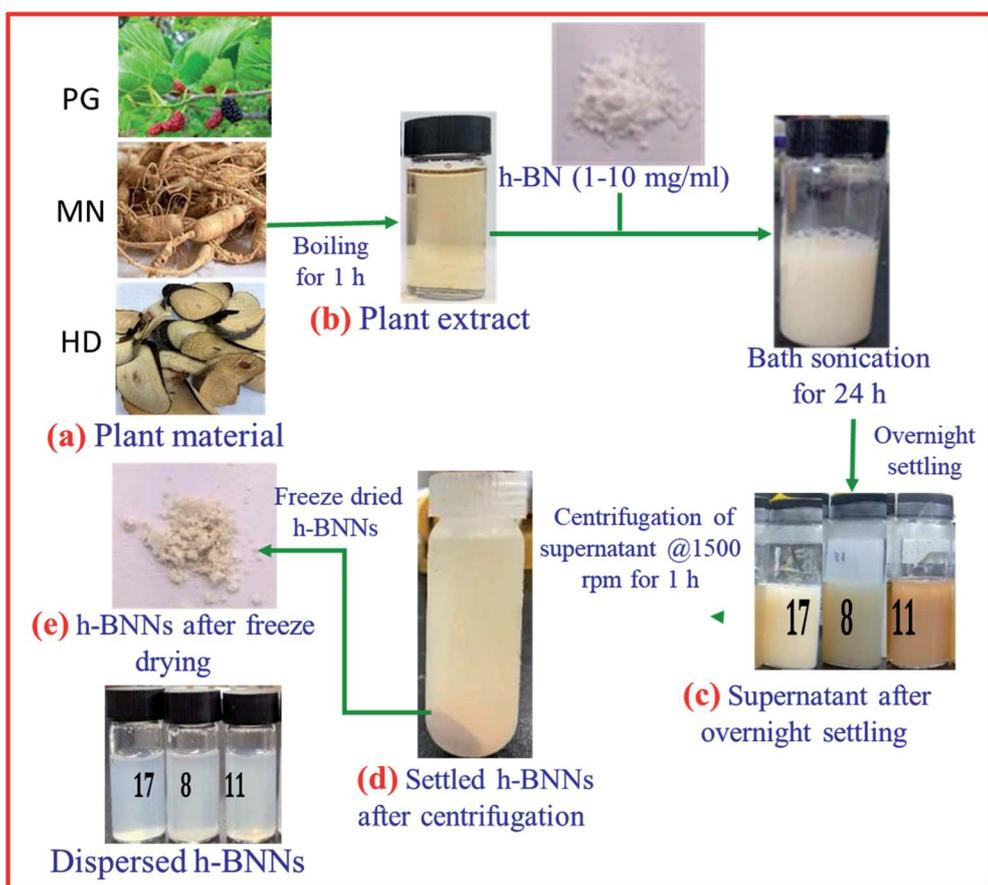
Fig. 16 A schematic diagram of a green exfoliation synthesis route using plant material extracts.<sup>153</sup>
