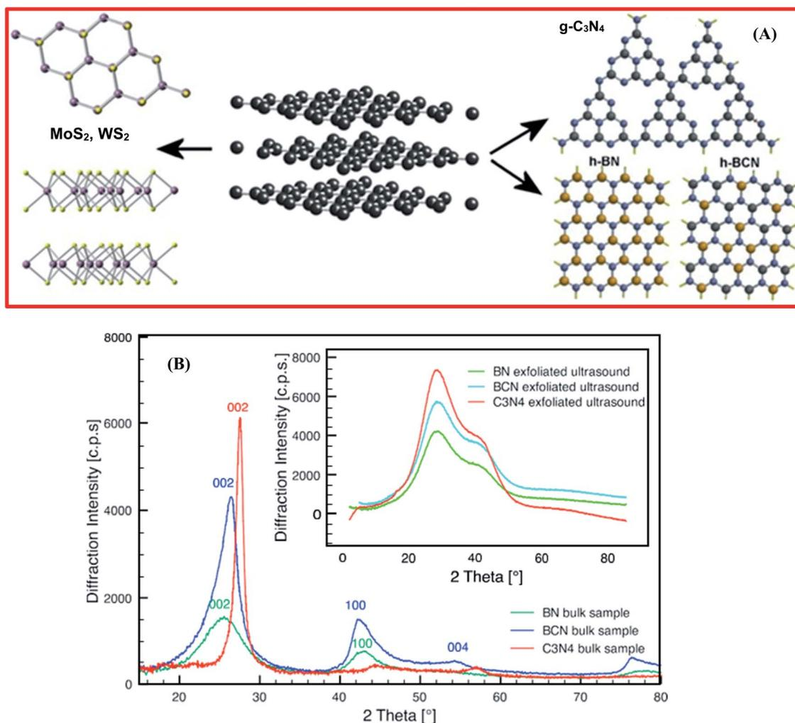
Fig. 5 (A) The exfoliated structures of inorganic analogues of graphene –  $\text{MoS}_2$ ,  $\text{WS}_2$ ,  $\text{g-C}_3\text{N}_4$ , h-BN, and h-BCN. (B) XRD patterns of bulk synthetic samples of h-BN, h-BCN, and  $\text{g-C}_3\text{N}_4$ . However, the inset shows the XRD patterns of the ultrasound-exfoliated samples.<sup>93</sup>
