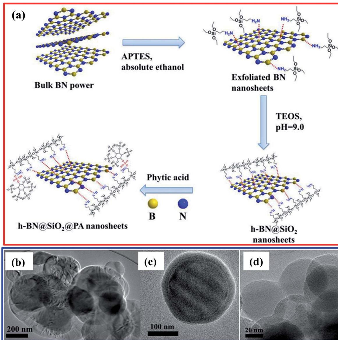
Fig. 26 (a) A schematic illustration of the synthesis of functionalized h-BN. (b) TEM images of bulk h-BN, (c) h-BN@SiO<sub>2</sub>, and (d) SiO<sub>2</sub> spheres.<sup>236</sup>
