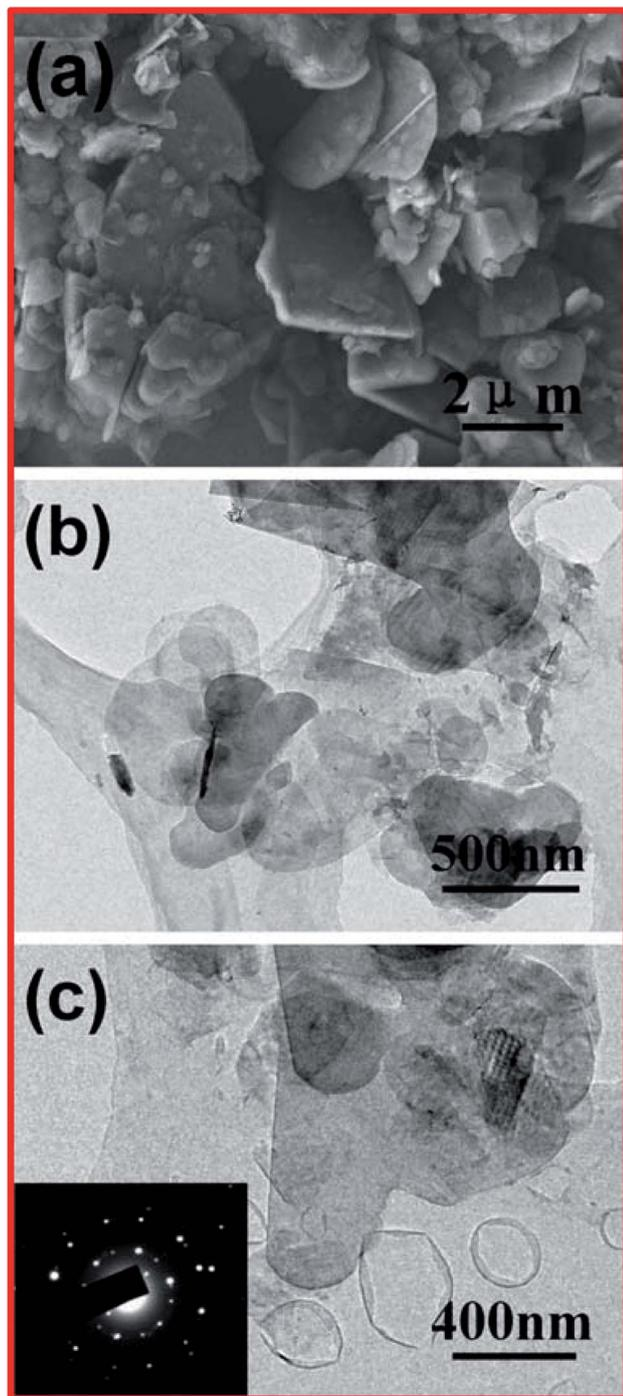
Fig. 4 (a) An SEM image of h-BN particles. (b) A TEM image of large-number BNNSs. (c) A TEM image of few-layered BNNSs; the inset shows the selected area electron diffraction (SAED) pattern.<sup>86</sup>
