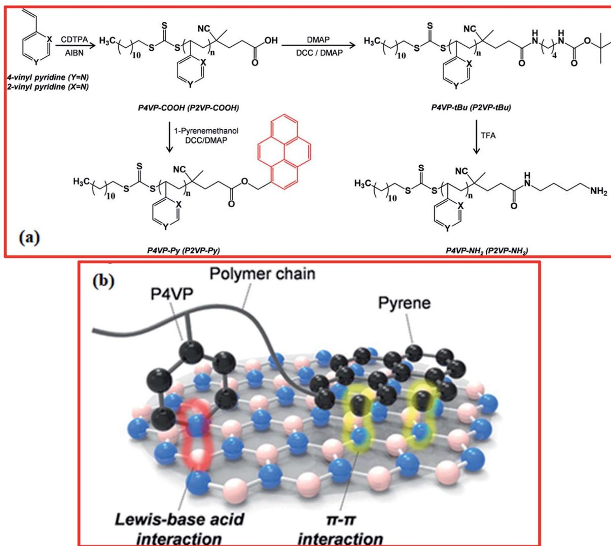
Fig. 27 (a) The reaction scheme for  $P_nVP$  ( $n = 2$  and  $4$ ) with different functional groups: carboxylic acid ( $P_nVP-COOH$ ), pyrene ( $P_nVP-Py$ ), *tert*-butyl ( $P_nVP-tBu$ ), and amine ( $P_nVP-NH_2$ ). (b) An illustration of the suggested mechanism for dual Lewis acid–base and  $\pi - \pi$  interactions using  $P_4VP-Py$  molecules on BN.<sup>237</sup>
