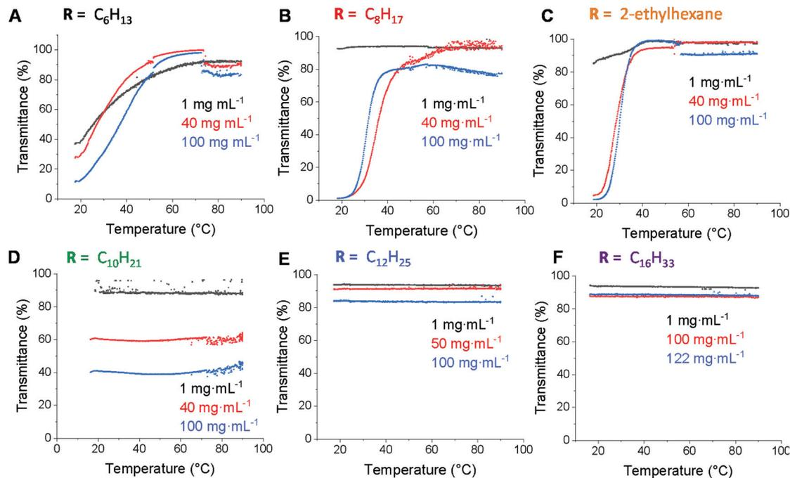
**Fig. 4** UV-Vis transmittance spectra as function of temperature and concentration in *n*-dodecane for poly( $\epsilon$ -allyl- $\epsilon$ -caprolactone) functionalised with (a) 1-hexanethiol, (b) 1-octanethiol, (c) 2-ethyl hexanethiol, (d) 1-decanethiol, (e) 1-dodecanethiol and (f) 1-hexadecanethiol (heating rate = 1 °C min<sup>-1</sup> from 20–95 °C).
