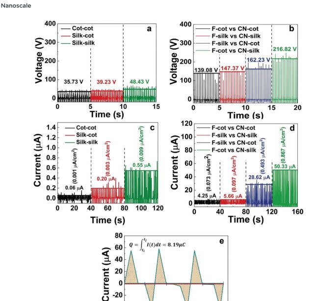
Fig. 6 (a) Output voltage of pristine-TENGs, (b) output voltage of N-TENGs, (c) output current of pristine-TENGs, (d) output current of N-TENGs and (e) three movement cycles of the  $I_{sc}$  signal of F-cot/CN-silk with the average calculated surface charge.
