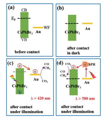
Fig. 14 (a) Band structure of CsPbBr $_3$  nanocrystals and Au nanoparticles before contact. (b) Fermi level alignment after their close contact in the dark. Schematic diagram of two excitation wavelength-dependent charge separation mechanisms in the CsPbBr $_3$ -Au nanocomposite under light irradiation with (c)  $\lambda$  >420 nm or (d)  $\lambda$  >580 nm. (a–d) Reprinted from ref. 194, Copyright 2021, with permission from Elsevier.
