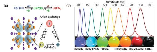
Fig. 5 (a) Schematic of the halide anion-exchange process. Reproduced with permission from ref. 38 at https://pubs.acs.org/doi/abs/10.1021/acs. nanolett.5b02404; further permissions are directed to the ACS. (b) Photoluminescence spectra and the corresponding photographs (under varied daylight and UV excitation) of colloid composition-tuned APbX<sub>3</sub> NCs. From ref. 92, reprinted with permission from AAAS.
