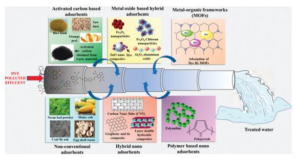
Fig. 17 Schematic presentation of water pollution from dye wastewater, their adsorptive removal using various adsorbents, and the production of treated water
