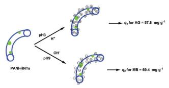
Fig. 15 Schematic illustration of PANI-HNTs at pH 3 and 9 (blue color: PANI-HNTs and green color: AG) [Reprinted with permission from ref. 275. Copyright 2018, The Royal Society of Chemistry].
