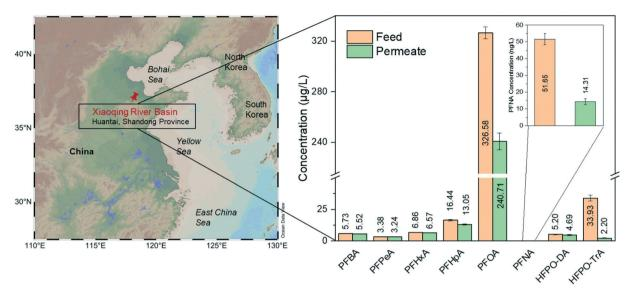
Fig. 5 Treatment of water sample from Xiaoging River basin by AM membrane. The map is generated from Schlitzer, Reiner, Ocean Data View, odv.awi.de, 2020. The removal efficiencies are summarized in the ESI† (Table S4).
