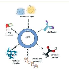
Fig. 10 A CQD (centre, core and shell) showing the different types of structures that can be bound to its shell.
