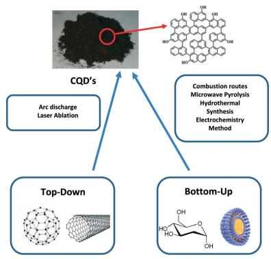
Fig. 4 A general scheme outlining how CQDs are generated from different successful top-down and bottom-up methods.<sup>29</sup> The top-down and bottom-up boxes display typical starting materials used for the methods shown in the boxes (centre). The top of the scheme shows the final CQD product and its general chemical structure.
