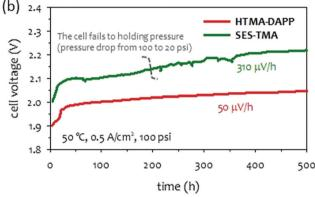
Fig. 16 (a) Stress-strain curves of HTMA-DAPP and SES-TMA AEMs. (b) Comparison of long-term performance of AEMWEs using HTMA-DAPP (78 μm thick) and SES-TMA (53 μm thick) AEMs. Ionomer: Aemeon, Co<sub>3</sub>O<sub>4</sub> (3 mg cm $^{-2}$ ), cathode: Pt black (3 mg $_{\rm Pt}$  cm $^{-2}$ ). The AEMWE cell data was produced at Nel Hydrogen.
