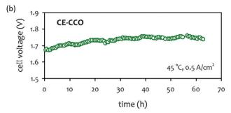
Fig. 15 (a) Catalyst degradation pathways under AEMWE operating conditions. (b) Durability of 1 M KOH-fed AEMWE at 500 mA cm<sup>-2</sup> at 45 °C. AEM: Sustainion® X37-50, anode: CuCo-oxide on nickel form (CE-CCO), cathode: Pt/C (1 mg<sub>Pt</sub> cm<sup>-2</sup>).<sup>92</sup> Adapted with permission.<sup>92</sup> Copyright 2020, Elsevier.
