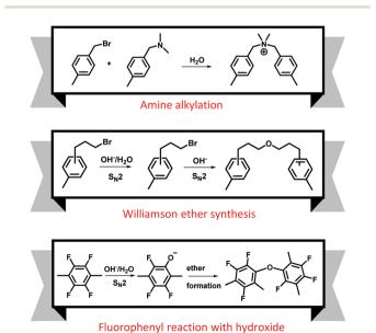
Fig. 14 Several cross-linking pathways of AEMs under high pH conditions.
