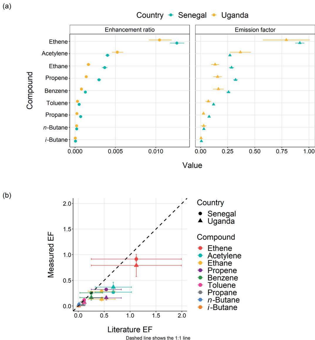
Fig. 5 (a) Enhancement ratio ( $\Delta\text{VOC}/\Delta\text{CO}$ ) and emission factor calculations for selected VOCs. (b) plot of measured against literature emission factors (taken from Andreae (2019)<sup>49</sup>). The dash line represents 1 : 1.
