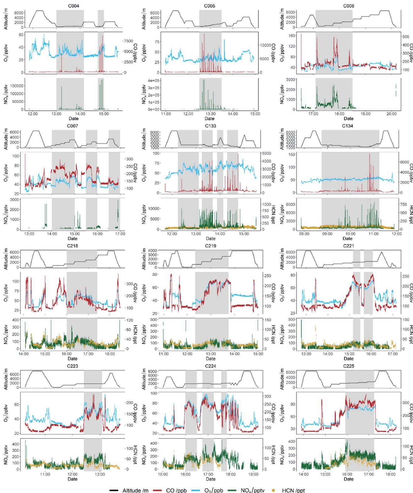
Fig. 3 Time series of NO<sub>x</sub>, HCN, altitude, O<sub>3</sub>, and CO for each flight. Grey shaded areas show when fire plumes were being sampled (see text for description of plume identification).
