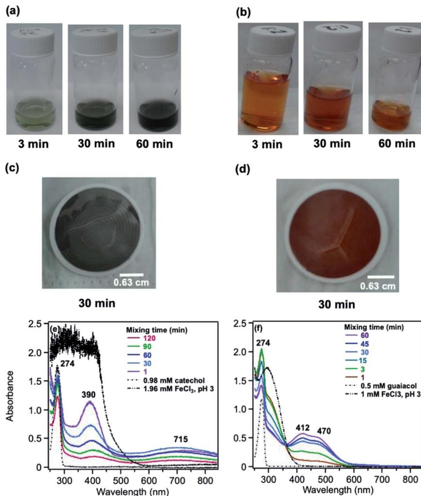
Fig. 6 Dark reaction of catechol and guaiacol with  $\text{FeCl}_3$  at pH 3: (a and b) digital images of the 1 : 2 organic reactant/Fe molar ratio of unfiltered solutions as a function of time; (c and d) particles on filter after 30 min; and (e and f) the corresponding UV-vis spectra after filtration. Reproduced from ref. 70 with permission from the American Chemical Society, © 2015.
