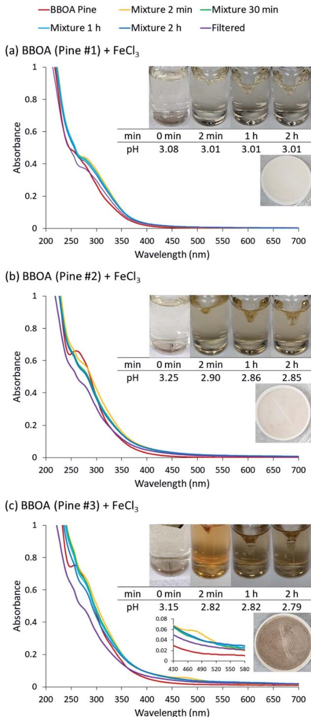
Fig. 20 UV-Vis absorption spectra of mixture of excess  $\text{Fe}(\text{III})$  and BBOA extracts. Different colors of traces correspond to the spectra of BBOA before mixing (red), 2 min after mixing (orange), 30 min after mixing (green), 1 h after mixing (light blue), 2 h after mixing (dark blue), and filtered solution (purple). Reproduced from ref. 190 under Creative Commons License (CC BY-NC) from the Royal Society of Chemistry, © The Author(s), 2021.
