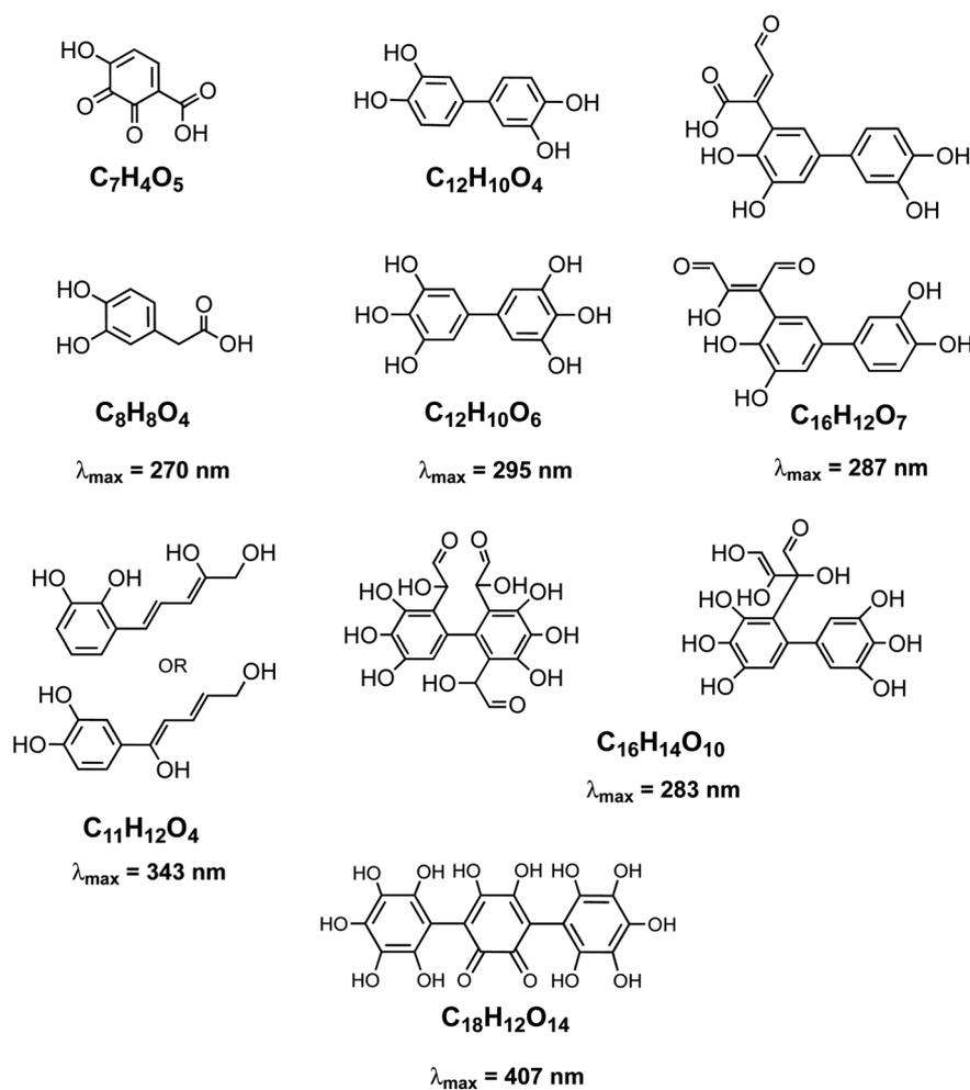
**Scheme 2** Structure of molecules and oligomers and their characteristic absorption wavelength detected in the reaction of catechol with Fe(III) under conditions characteristic of viscous multicomponent aerosol systems with relatively high ionic strength ( $I = 1\text{--}12 \text{ m}$ ) and acidic pH ( $\sim 2$ ) using UHPLC-MS. Modified from ref. 148 with permission from The American Chemical Society, © 2021.
