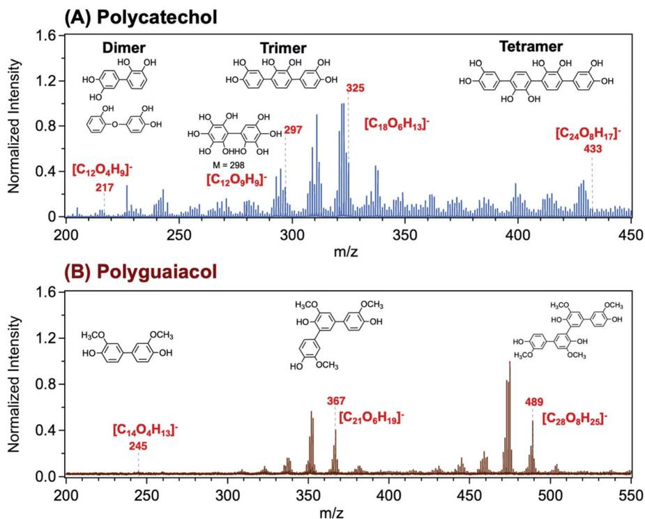
Fig. 8 Representative MALDI-TOF mass spectrum of (A) polycatechol and (B) polyguaiacol thin films in the negative ion reflector mode,  $[M-H]^-$ . The structure of fragments was based on ref. 207 for polycatechol and ref. 208 for polyguaiacol. No additional matrix compound was used in the spectra collection. Spectra were collected with the assistance of Dr Lauren T. Fleming, Prof. Sergey A. Nizkorodov, and Dr Ben Katz at the University of California Irvine Mass Spectrometry Facility.
