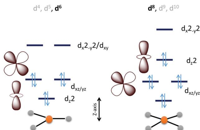
Scheme 2 An electronic structure consideration of  $CO_2$  activation and reduction using a 3d metal active site having trigonal (left) and tetragonal (right) ligand field.
