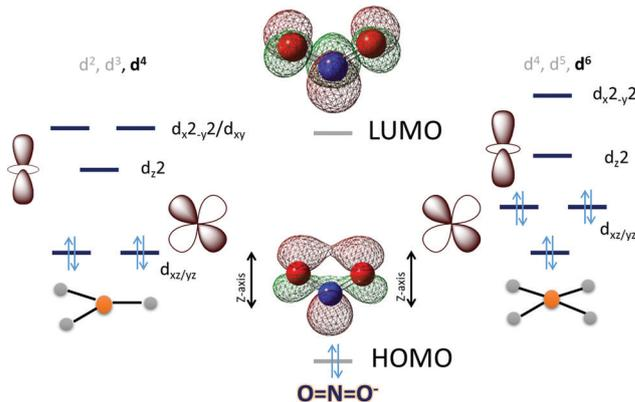
Scheme 3 An electronic structure consideration of NO<sub>2</sub><sup>-</sup> activation and reduction using a 3d metal active site having trigonal (left) and tetragonal (right) ligand field.
