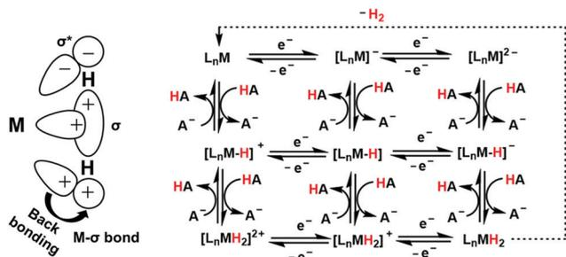
Scheme 25 Schematic presentation of the formation of M–H<sub>2</sub> σ bond and M<sub>dπ</sub> → H<sub>2</sub> backdonation (left). Possible mechanistic pathways for catalytic reduction of proton to hydrogen in the natural hydrogenases or synthetic catalysts (right).
