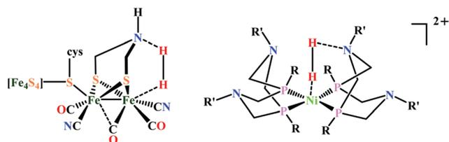
Fig. 35 [FeFe]-hydrogenase active site (left) and [Ni(P<sup>R</sup><sub>2</sub>N<sup>R'</sup><sub>2</sub>)<sub>2</sub>]<sup>2+</sup> molecular catalyst (right), H<sub>2</sub> bound in each case in the active site.
