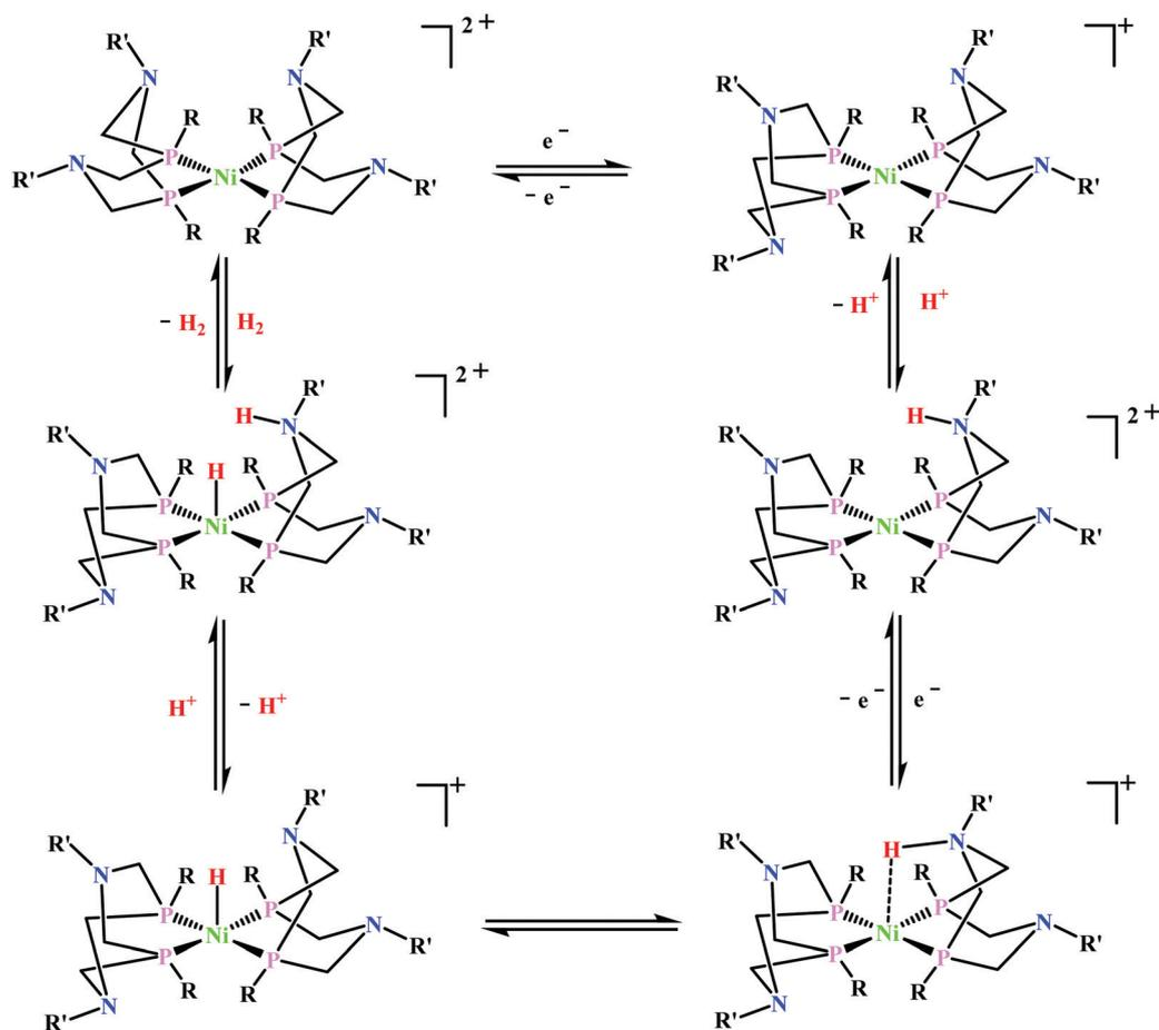
Scheme 35 H<sub>2</sub> oxidation (counter-clockwise) and evolution (clockwise) cycle mediated by  $[\text{Ni}(\text{P}^{\text{R}}_2\text{N}^{\text{R}'}_2)]^{2+}$  molecular catalysts.<sup>548</sup> This cycle is a simplification that neglects certain side reaction pathways, and the order of the steps depends on the identities of substituents R and R'.<sup>428</sup>
