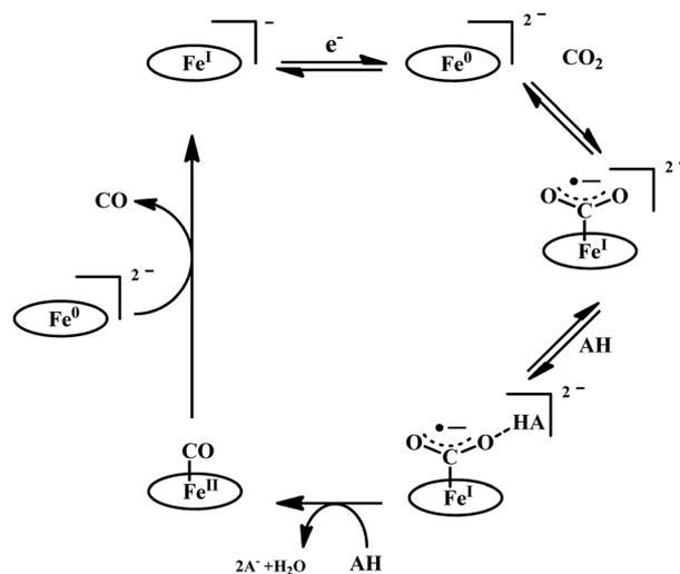
Scheme 7 Proposed mechanistic pathway for the reduction of CO<sub>2</sub> to CO by Fe-porphyrin electrocatalysts.
