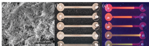
Fig. 1 (a) SEM of aerogel of C/CdTe-GOx, (b) microchannel sensor under incandescent lamp, (c) microchannel sensor under ultraviolet lamp.
