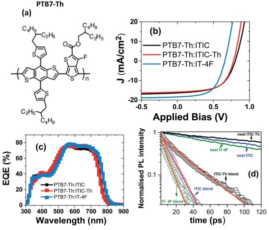
Fig. 4 Device characteristics of PTB7-Th:NFAs (ITIC, ITIC-Th and IT-4F) blends: (a) molecular structure of PTB7-Th, (b) current density-voltage (J-V) curves, (c) external quantum efficiency (EQE) of devices, (d) PL decays in the blends of electron acceptors with PTB7-Th which were used to make solar cells (symbols) and in neat electron acceptor films (solid lines). Solid red lines are the fits using eqn (4) which were used to estimate the average domain sizes of acceptors
