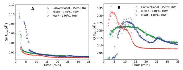
Fig. 5 (A) Sn atomic displacement parameters ( $U_{iso}$ ) for conventional (green), mixed (red), and MWR-only (blue) synthesis conditions. (B) O  $U_{iso}$  values for the same reaction conditions shown in (A). the presence of multiple peaks in O  $U_{iso}$  during MWR-assisted reactions indicates changes on the oxygen sublattice not present during conventional hydrothermal conditions.
