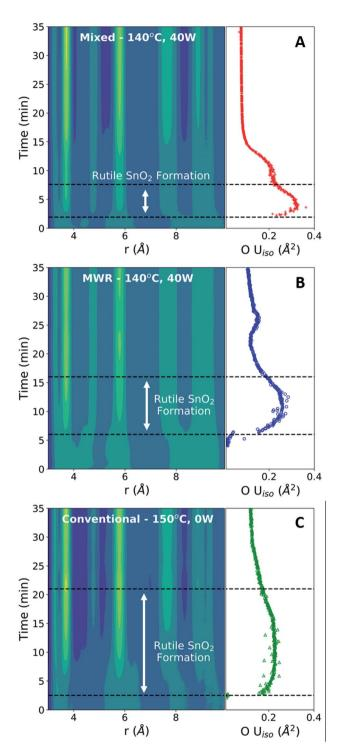
Fig. 6 Contour plots of mixed (A), MWR-only (B), and conventional (C) synthesis conditions compared with O  $U_{\rm iso}$  during the same time period. Sharper peaks in the displacement parameter are observed during MWR-assisted synthesis and correspond to an increase in intensity of the first two Sn-Sn peaks. Conventional synthesis results in a broad, lower-intensity peak in  $U_{iso}$  which exists throughout over half the total reaction time.
