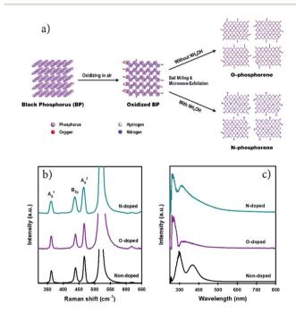
Fig. 1 (a) Schematic illustration for the preparation of N-doped and O-doped phosphorene using a combination of ball milling and microwave-assisted LPE methods. (b) Raman (on a silicon (Si) substrate) and (c) UV-vis spectra of non-doped, O-doped and N-doped phosphorene.
