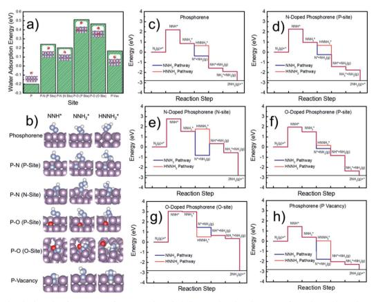
Fig. 6 (a) Calculated adsorption free energy of water at six typical sites on the phosphorene surfaces. Insets show the optimized water adsorption geometries. (b) Optimized structures of NNH\*, NNH\*, and HNNH\*, species adsorbed at the six typical sites. (c-h) Calculated free energy pathways of the NRR at six typical sites on the phosphorene surfaces. Purple, blue, white, and red spheres represent P, N, H, and O, respectively.
