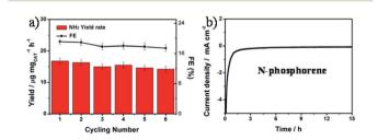
Fig. 4 (a) Cycling stability results of N-phosphorene at 0 V vs. RHE. (b) Long-term durability test with chronoamperometry of N-phosphorene toward the electrocatalytic NRR in a N2-saturated 0.1 M KOH solution for 15 h at 0 V vs. RHE
