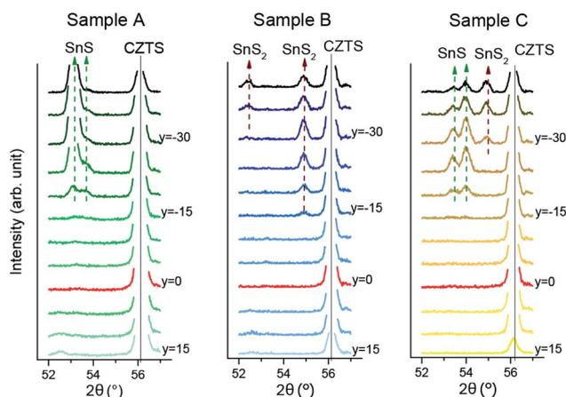
**Fig. 4** XRD patterns of samples A, B and C in a  $2\theta$  range with expected SnS and  $\text{SnS}_2$  reflections. *y* denotes the distance to the Cu/Sn = 2 line in mm.
