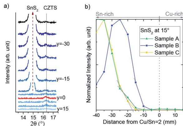
**Fig. 3** (a) XRD patterns in regions with  $\text{SnS}_2$  reflection at 15° for different positions parallel to the Cu/Sn = 2 line on sample B. *y* denotes the distance to the Cu/Sn = 2 line in mm. (b) Integrated intensity of the reflection at 15°. The dotted lines are guides to the eye for the interpolation to the phase boundary.
