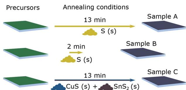
Fig. 1 Sample overview illustrating the different processing conditions during the annealing step in terms of annealing time and atmosphere. The annealing temperature is 550 °C.
