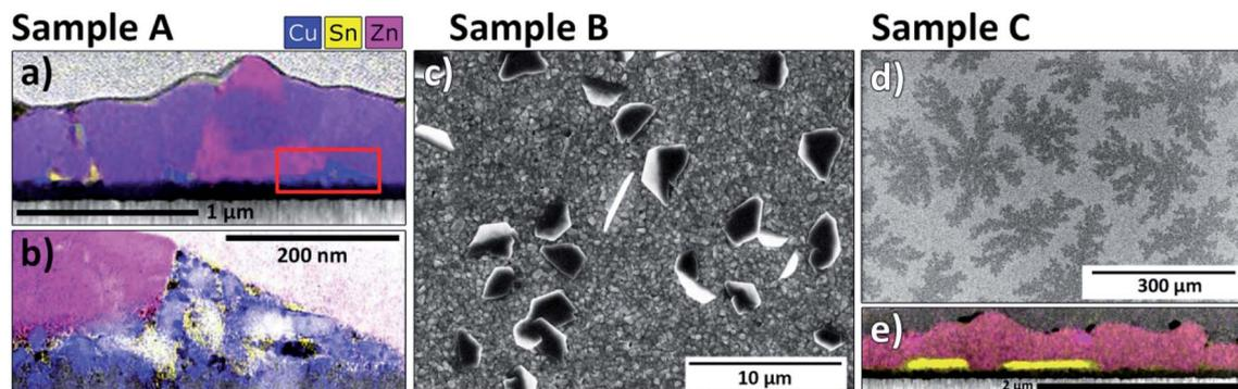
Fig. 8 Observation of  $\text{SnS}_x$  secondary phases in samples A, B and C. Sample A: STEM and EDX images, (a) with Cu (blue), Zn (pink) and Sn (yellow) and (b) close-up image of area marked with red rectangle. Sample B: (c) top view SEM with  $\text{SnS}_x$  flakes visible on surface. Sample C: (d) top view SEM with dendrite structures. (e) STEM and EDX image with Sn (yellow) and Zn (magenta).
