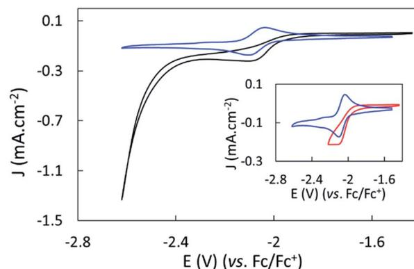
Fig. 2 Cyclic voltammograms of complex **1** under Ar (blue) and CO<sub>2</sub> applying potentials from -1.52 V to -2.22 V vs. Fc/Fc<sup>+</sup> (red, inset) and from -1.52 V to -2.62 V vs. Fc/Fc<sup>+</sup> (black). 1 mM solution in dry CH<sub>3</sub>CN containing 0.1 M TBAPF<sub>6</sub> electrolyte; GC working electrode; The scan rate was 50 mV s<sup>-1</sup>; the second scan is shown.
