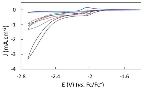
Fig. 3 Cyclic voltammograms of 1 mM complex **1** with 0.1 M TBAPF<sub>6</sub> in dry CH<sub>3</sub>CN on a GC electrode under Ar (blue), CO<sub>2</sub> (red), CO<sub>2</sub> with 0.1 M TFE (black), CO<sub>2</sub> with 0.1 M H<sub>2</sub>O (green) and CO<sub>2</sub> with 0.1 M PhOH (purple). The scan rate was 50 mV s<sup>-1</sup>; the second scan is shown.
