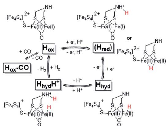
**Scheme 1** Schematic representation of the catalytic cycle of  $[\text{FeFe}]$ -hydrogenase, based on the states observed under whole-cell conditions including the protonated hydride species ( $\text{H}_{\text{hyd}}\text{H}^+$ ). The catalytic cycle is derived from ref. 10 and 29, and the debated  $\text{H}_{\text{red}}$  state is shown in parenthesis together with two proposed structures (protonated on the ligand or metal, respectively).
