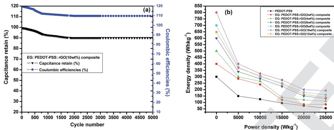
Fig. 12 (a) Capacitance retention (%) and coulombic efficiency (%) over 5000 cycles at constant current density ( $1 \text{ A g}^{-1}$ ), (b) energy density versus power density (Ragone plot) for all the composite thin films.
