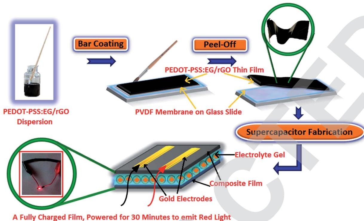
Fig. 2 Schematic representation of flexible electrode fabrication.
