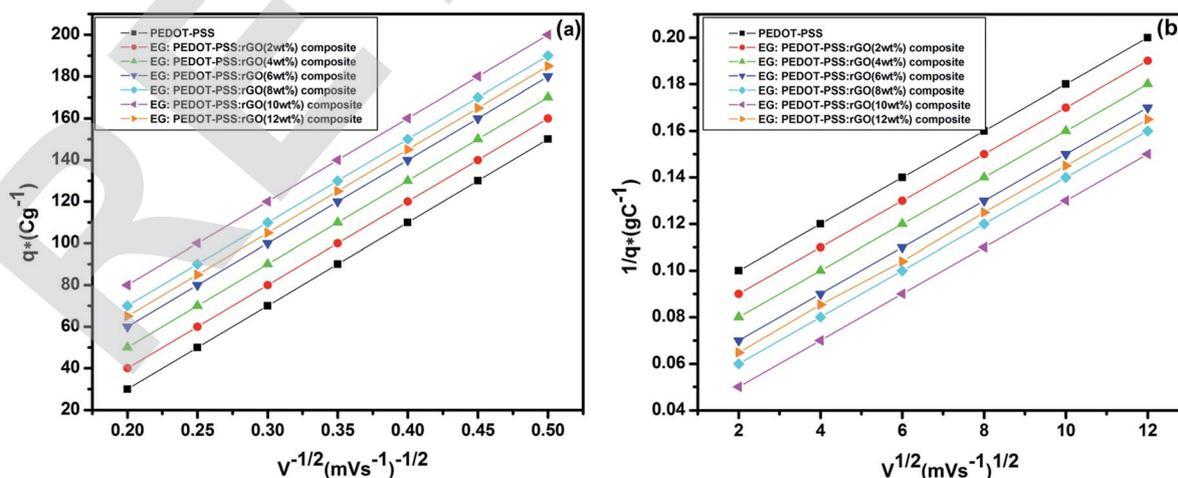
Fig. 8 Dependence of (a) voltammetric charge ( $q^*$ ) with inverse square root of scan rate ( $V^{-1/2}$ ) and (b) dependence of inverse voltammetric charge ( $1/q^*$ ) with square root scan rate ( $V^{1/2}$ ).
